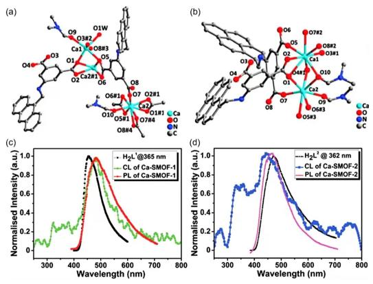
Fig. 4 The coordination configuration of Ca1 and Ca2 for Ca-SMOF 1 (a) and Ca-SMOF 2 (b). The CL and PL spectra of Ca-SMOF 1 (c) and Ca-SMOF 2 (d), along with the spectra of their respective free ligands,  $H_2L^2$  and  $H_2L^2$ . Reprinted with permission.<sup>53</sup> Copyright 2019, Royal Society of Chemistry.
