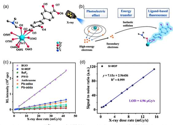
**Fig. 8** (a) The coordination environment of Sr<sup>2+</sup> centers in **Sr-MOF**. (b) Diagram of the RL mechanism of **Sr-MOF**. (c) The linear relationship between RL intensity and X-ray dose rates of **Sr-MOF**, BGO, PWO, BaF<sub>2</sub>, organic crystal anthracene and reported Pb-based SMOFs (**Pb-adba**<sup>60</sup> and **Pb-adda**<sup>61</sup>). (d) The detection limit is Sr-MOF. <sup>59</sup> Copyright 2023, Royal Society of Chemistry. Reprinted with permission. <sup>59</sup>
