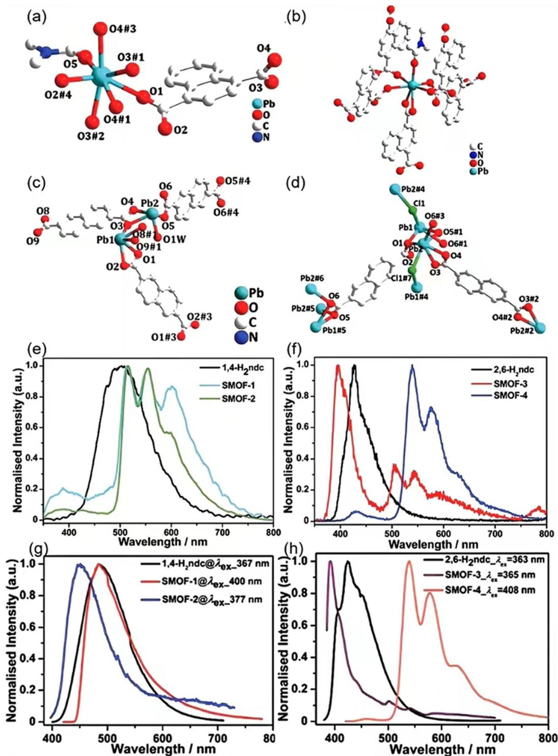
Fig. 10 Pb(II) coordination within Pb-SMOF-1 (a), Pb-SMOF-2 (b), Pb-SMOF-3 (c), Pb-SMOF-4 (d). The XSL spectra of 1,4-H<sub>2</sub>ndc, Pb-SMOF-1 and Pb-SMOF-2 (e) and 2,6-H<sub>2</sub>ndc, SMOF-3 and SMOF-4 (f). The peak steady-state PL spectra of free 1,4-H<sub>2</sub>ndc and Pb-SMOFs 1–2 (g), and 2,6-H<sub>2</sub>ndc and Pb-SMOFs 3–4 (h). Reprinted with permission.<sup>64</sup> Copyright 2019, Royal Society of Chemistry.
