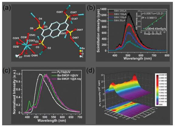
Fig. 17 (a) The coordination environments of PyTS<sup>4-</sup> ligand and Ba<sup>2+</sup> ions in **Ba-SMOF**. (b) XSL spectra with X-ray dosage rate detection performance inset. (c) Solid-state photoluminescent spectra for free ligands Na<sub>4</sub>PyTS and Ba-SMOF, along with XSL spectra for Ba-SMOF. (d) Solid-state synchronization fluorescence spectra for Ba-SMOF with gradient scanning step of 5 nm. Reprinted with permission.<sup>71</sup> Copyright 2024, Wiley.
