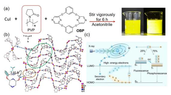
Fig. 2 (a) The preparation method of **Cu-MOF 1-rod**. (b) Crystal structure of **Cu-MOF 1**. (c) Scintillation mechanism of the detector. Reprinted with permission. <sup>51</sup> Copyright 2023, Wiley.
