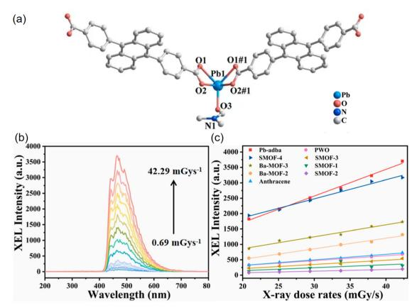
Fig. 11 (a) Coordination environments of the Pb<sup>2+</sup> ion. (b) The XEL spectra in the dose rate range of 0.69–42.29 mGy s<sup>-1</sup> at a voltage of 50 kV. (c) Linear correlation between XEL intensity and dose rate for Pb-adba, PWO, anthracene crystals, and other documented scintillating MOFs. Reprinted with permission.<sup>60</sup> Copyright 2022 Elsevier.
