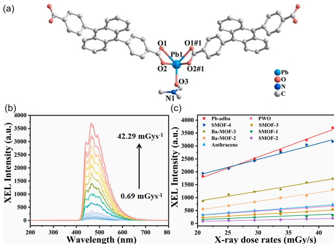
Fig. 11 (a) Coordination environments of the  $\text{Pb}^{2+}$  ion. (b) The XEL spectra in the dose rate range of 0.69–42.29  $\text{mGy s}^{-1}$  at a voltage of 50 kV. (c) Linear correlation between XEL intensity and dose rate for **Pb-adba**, PWO, anthracene crystals, and other documented scintillating MOFs. Reprinted with permission.<sup>60</sup> Copyright 2022 Elsevier.
