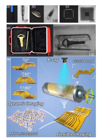
Fig. 21 (a)-(c) Visual representations of imaging for a ballpoint pen, sunflower kernel, and microchip; (d) Depicting a mock security inspection process with the scintillator screen; (e) Dynamic flexible X-ray imaging system and real-time imaging photographs of circuit boards. Reprinted with permission from ref. 51. Copyright 2023, Wiley.
