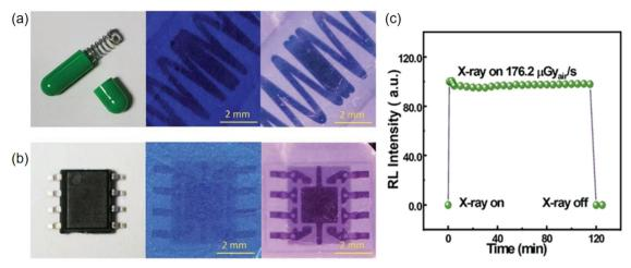
Fig. 19 X-ray imaging of  $Cs_3Cu_2l_5$ : In. (a) a spring in a capsule shell and (b) a small electronic component using undoped  $Cs_3Cu_2l_5$  (in the middle) and In<sup>+</sup>-doped Cs<sub>x</sub>Cu<sub>2</sub>I<sub>s</sub> (on the right) SCs. (c) The RL intensity of the Cs<sub>x</sub>Cu<sub>2</sub>I<sub>s</sub>-PSS screen is directly proportional to the X-ray dose rate. Reprinted with permission.<sup>54</sup> Copyright 2022, Wiley.
