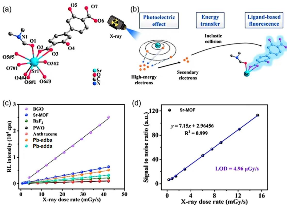
Fig. 8 (a) The coordination environment of  $\text{Sr}^{2+}$  centers in **Sr-MOF**. (b) Diagram of the RL mechanism of **Sr-MOF**. (c) The linear relationship between RL intensity and X-ray dose rates of **Sr-MOF**, BGO, PWO,  $\text{BaF}_2$ , organic crystal anthracene and reported Pb-based SMOFs (**Pb-adba**<sup>60</sup> and **Pb-adda**<sup>61</sup>). (d) The detection limit is Sr-MOF.<sup>59</sup> Copyright 2023, Royal Society of Chemistry. Reprinted with permission.<sup>59</sup>
