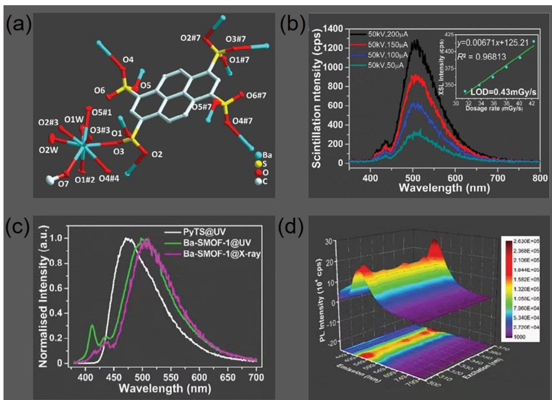
Fig. 17 (a) The coordination environments of  $PyTS^{4-}$  ligand and  $Ba^{2+}$  ions in **Ba-SMOF**. (b) XSL spectra with X-ray dosage rate detection performance inset. (c) Solid-state photoluminescent spectra for free ligands  $Na_4PyTS$  and **Ba-SMOF**, along with XSL spectra for **Ba-SMOF**. (d) Solid-state synchronization fluorescence spectra for **Ba-SMOF** with gradient scanning step of 5 nm. Reprinted with permission.<sup>71</sup> Copyright 2024, Wiley.
