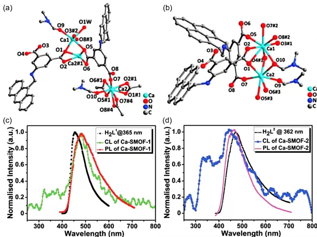
Fig. 4 The coordination configuration of Ca1 and Ca2 for **Ca-SMOF 1** (a) and **Ca-SMOF 2** (b). The CL and PL spectra of **Ca-SMOF 1** (c) and **Ca-SMOF 2** (d), along with the spectra of their respective free ligands,  $\text{H}_2\text{L}^1$  and  $\text{H}_2\text{L}^2$ . Reprinted with permission.<sup>53</sup> Copyright 2019, Royal Society of Chemistry.
