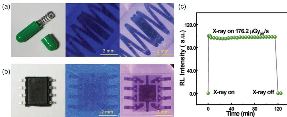
Fig. 19 X-ray imaging of  $\text{Cs}_3\text{Cu}_2\text{I}_5:\text{In}$ . (a) a spring in a capsule shell and (b) a small electronic component using undoped  $\text{Cs}_3\text{Cu}_2\text{I}_5$  (in the middle) and  $\text{In}^+$ -doped  $\text{Cs}_3\text{Cu}_2\text{I}_5$  (on the right) SCs. (c) The RL intensity of the  $\text{Cs}_3\text{Cu}_2\text{I}_5$ -PSS screen is directly proportional to the X-ray dose rate. Reprinted with permission.<sup>54</sup> Copyright 2022, Wiley.
