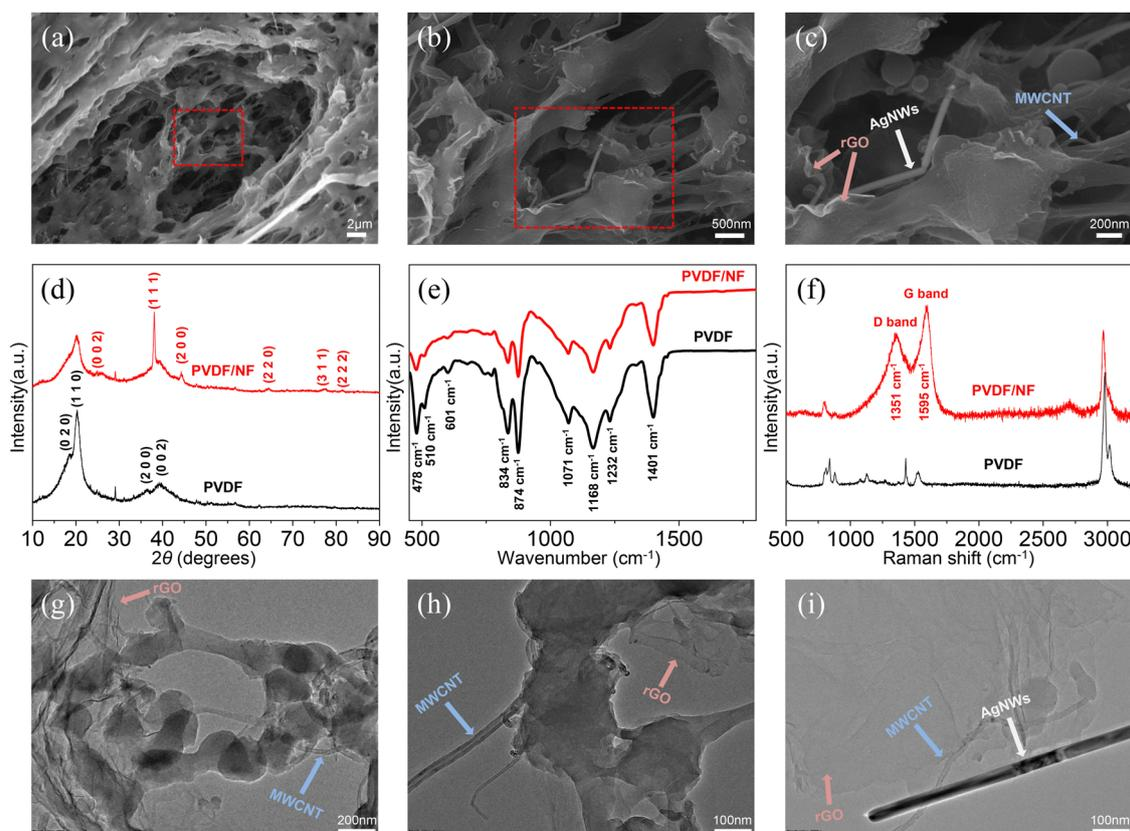
Fig. 2 Characterization of the PVDF/NF ink: (a)–(c) SEM images of PVDF/NF at magnifications of  $\times 10k$ ,  $\times 50k$ , and  $\times 100k$ , respectively, (d) XRD patterns comparing PVDF and PVDF/NF, (e) FTIR spectra of PVDF and PVDF/NF, (f) Raman spectroscopy data for PVDF and PVDF/NF, and (g)–(i) TEM images of PVDF/NF.
