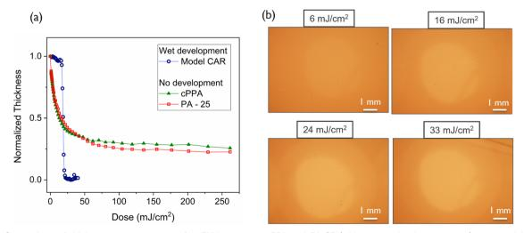
Fig. 3 (a) Comparison of thickness contrast curves after EUV exposure; cPPA and PA-25 (without any development step) to a model CAR after application of PEB and wet development (taken from ref. 7). (b) Optical image of EUV exposure points on the PA-25 coated wafer, the spot with exposure shows a decrease in thickness after spontaneous development after EUV exposure.
