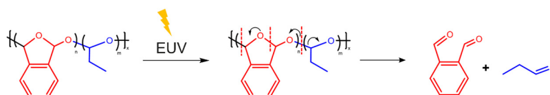
Fig. 5 Proposed EUV induced depolymerization of PA-25.
