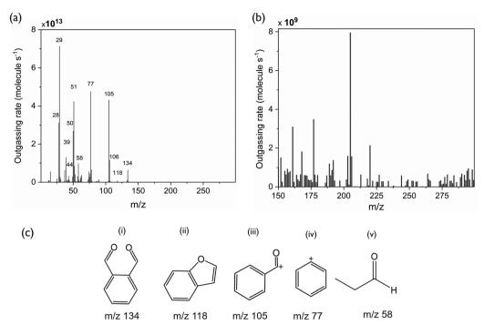
Fig. 4 (a) Mass spectra of outgassing species during EUV exposure of PA-25. (b) Zoomed-in view of peaks present at higher m/z (>150). (c) Molecular structure of major fragments of phthaldehyde and propanal.
