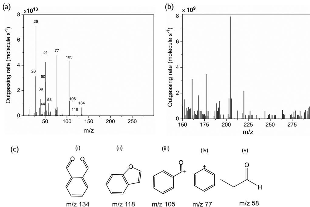
Fig. 4 (a) Mass spectra of outgassing species during EUV exposure of PA-25. (b) Zoomed-in view of peaks present at higher  $m/z$  ( $>150$ ). (c) Molecular structure of major fragments of phthalaldehyde and propanal.
