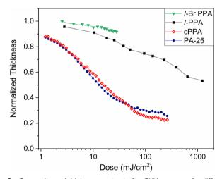
Fig. 2 Comparison of thickness contrast after EUV exposure for different PPA derivatives: l-Br PPA (green – with PEB and IPA development) & l-PPA (black without any development step) adapted from ref. 1 and 20. cPPA (red) and PA-25 (violet) used in this study are at least two orders of magnitude more sensitive than other two derivatives.
