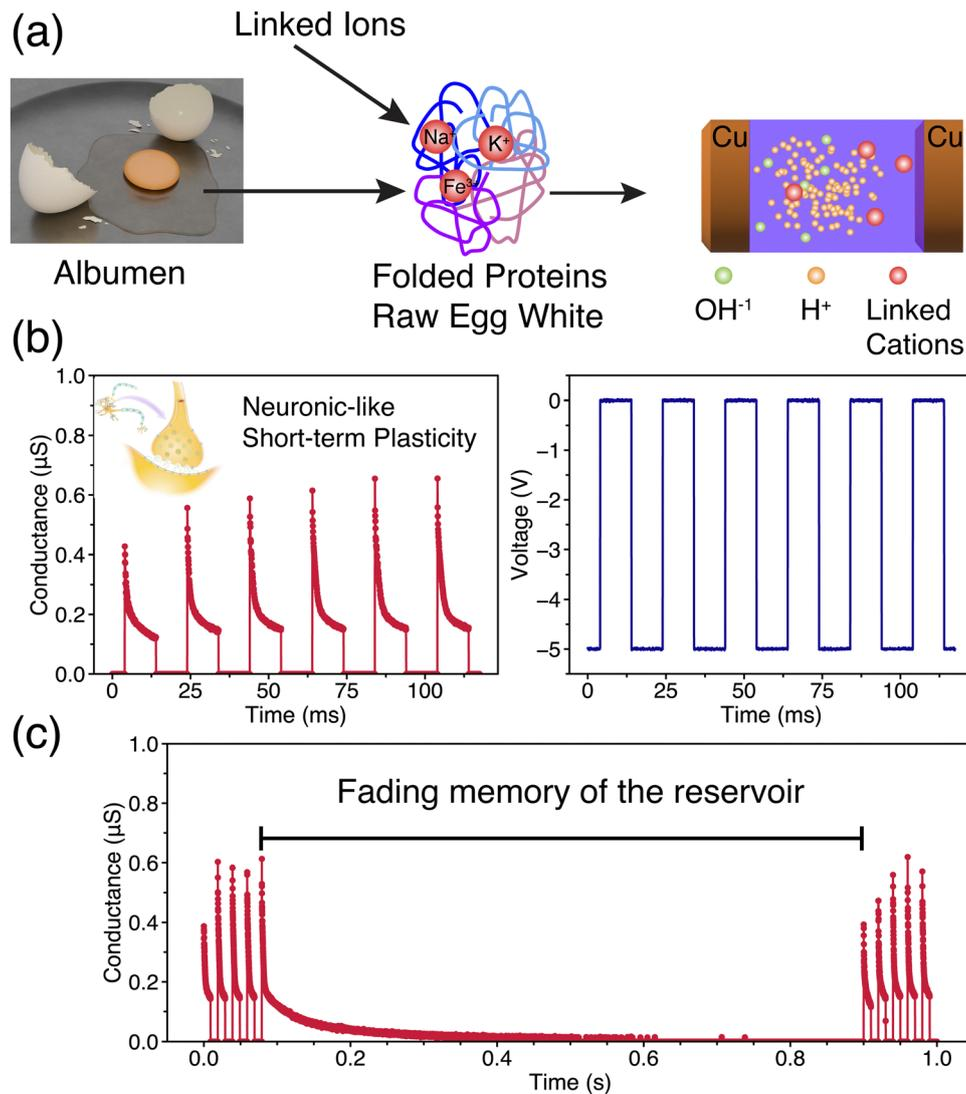
Fig. 2 (a) Idealization of the biological reservoir. The presence of a high concentration of ions bound to folded proteins in raw egg white creates an ionic fluid ideal for memory and resistivity switching behavior. (b) Neuromorphic behavior of the reservoir exhibits short term plasticity due to  $-5$  V, 10 ms pulses. Illustration of the biological synapse was adapted from ref. 41. (c) Illustration of the fading memory of the reservoir.
