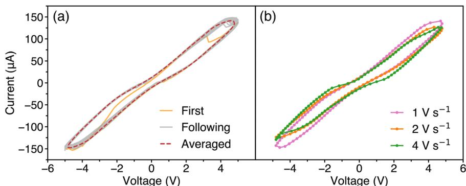
Fig. 1 Current–voltage characteristics of the reservoir for (a) 100 sweeps at a scan rate of  $1\text{ V s}^{-1}$  and (b) averaged 100 sweeps at scan rates of  $1\text{ V s}^{-1}$ ,  $2\text{ V s}^{-1}$ , and  $4\text{ V s}^{-1}$ .
