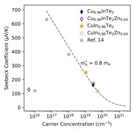
Fig. 6 Pisarenko analysis fit using an SPB model for the samples with carrier concentration over 10<sup>19</sup> holes cm<sup>-3</sup> extracts an effective mass of 0.8m<sub>e</sub>. The low carrier concentration sample does not fit with this trend, further confirming our suspicions of minority carrier contributions to Seebeck coefficient and carrier concentration. Literature data included from ref. 14
