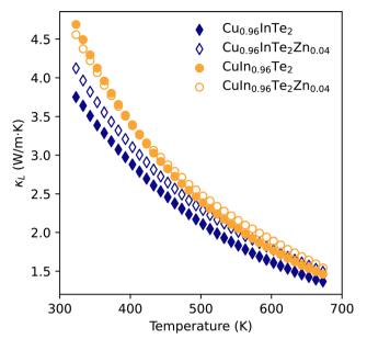
Fig. 8 Lattice thermal conductivity shows a marked decrease with increasing temperature, indicative of phonon–phonon scattering. Indeed, changing the defect concentrations leads to minimal differences in the lattice thermal conductivity.
