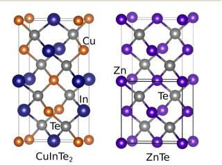
Fig. 1 The chalcopyrite-structured CuInTe<sub>2</sub> (left) forms a solid solution with zinc blende structured ZnTe (right). A single unit cell of ZnTe is shown with darkened boundaries.
