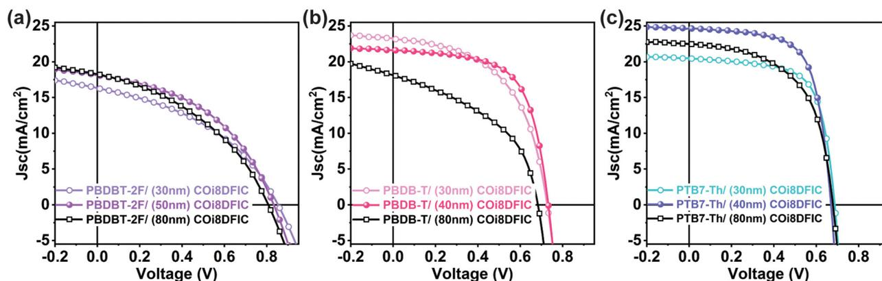
Fig. 2 Typical  $J-V$  characteristics of bilayer organic solar cells under simulated AM1.5G ( $100 \text{ mW cm}^{-2}$ ) illumination conditions with different acceptor layer thicknesses (a) PBDB-T-2F/COi8DFIC, (b) PBDB-T/COi8DFIC, and (c) PTB7-Th/COi8DFIC respectively.
