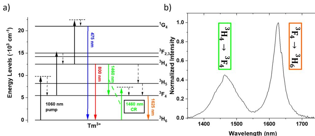
Fig. 2 (a) Energy level diagram of  $\text{Tm}^{3+}$  illustrating the photon-avalanche process under 1060 nm excitation. (b) Near-infrared emission spectrum of studied material under 1060 nm excitation.
