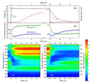
Fig. 5 (a) Transient EL emission (red) from OLED1 under application of the square-wave pulse bias (black) of +12 V (pulse width of  $15 \mu s$ ). (b) Transient ESFG intensities of OLED1 at the visible wavelengths of 650 (green) and 550 nm (blue). Time-resolved ESFG intensity variations in the visible excitation wavelength region of 460-670 nm for the OLED1 (c) turn-on and (d) turn-of.
