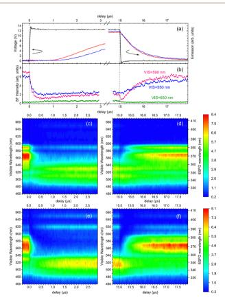
Fig. 6 (a) Transient EL emission from OLED2 (red) and OLED3 (blue) under application of the square-wave pulse bias (black) of +12 V (pulse width of 15  $\mu$ s). (b) Transient ESFG intensities of OLED2 at the visible wavelengths of 650 (green), 590 (pink), and 550 nm (blue). Time-resolved ESFG intensity variations of the OLED2 (c) turn-on and (d) turn-off. Timeresolved ESFG intensity variations of the OLED3 (e) turn-on and (f) turn-off.
