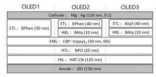
Fig. 1 Schematic of the structure of the three bottom-emission OLEDs fabricated in this study
