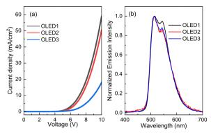
Fig. 2 (a) J-V characteristics of three OLED devices (OLED1, OLED2, and OLED3) used in this study. (b) Emission spectra of each OLED device at a current level of 0.15 mA. Emission intensities are normalized to the intensity at 515 nm.
