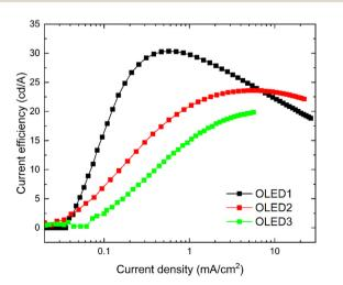
**Fig. 8** Current efficiencies of the three OLED devices. Note that the luminance measurements are only taken from the front of the devices, so they are not external quantum efficiencies.
