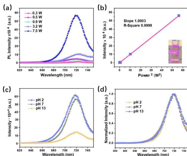
Fig. 5 Two-photon PL of QDs under 808-nm laser. (a) Two-photon spectra with different laser excitation intensities at 808 nm. (b) Relationship between the two-photon emission intensity and the square of laser power. Two-photon spectra (c) and normalized spectra (d) at different pH values.
