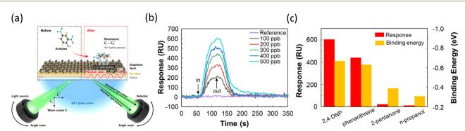
Fig. 10 (a) Schematic of the detection of 2,4DNP on a graphene-based SPR sensor. (b) Real-time SPR responses for 2,4 DNP at different concentrations ranging from 100 to 500 ppb. (c) Responses and calculated binding energies for various impurities. Reproduced with permission from ref. 77 Copyright@2024, John Wiley & Sons
