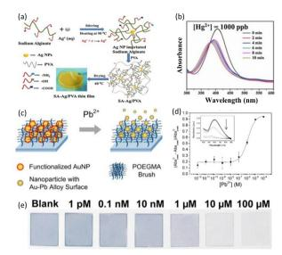
**Fig. 8** (a) Schematic of the SA–Ag composite thin film for  $Hg^{2+}$  sensing. (b) LSPR peak of the SA–Ag composite in an aqueous solution of 1000 ppb of  $Hg^{2+}$ . Reproduced with permission from ref. 58 Copyright©2017, Elsevier B. V. (c)  $Pb^{2+}$  sensing mechanism of functionalized AuNPs. (d) Responses and (e) photograph to various concentrations of  $Pb^{2+}$  ranging from 1 pM to 100 μM. Reproduced with permission from ref. 59 Copyright©2013, the American Chemical Society.
