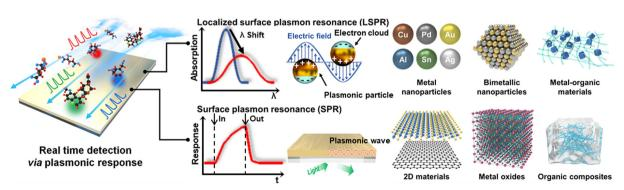
Fig. 1 Schematic of two representative technologies (LSPR and SPR) used in real-time detection via plasmonic reactions and the materials used for each technology
