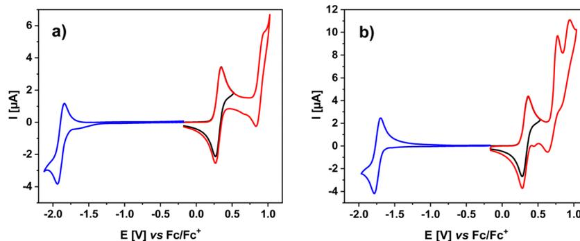
Fig. 2 Cyclic voltammograms of **4** (a) and **5** (b). Concentration of the studied compounds:  $1 \times 10^{-3}$  M, electrolyte: 0.1 M  $\text{Bu}_4\text{NPF}_6$  solution in DCM; scan rate:  $50 \text{ mV s}^{-1}$ .
