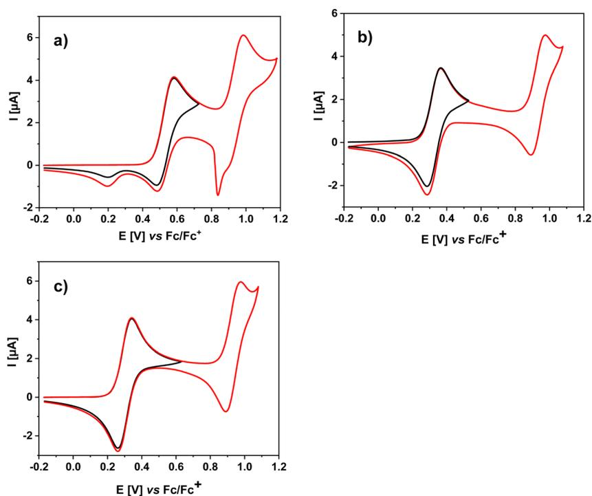
Fig. 1 Cyclic voltammograms of **1** (a), **2** (b) and **3** (c). Concentration of the studied compounds:  $1 \times 10^{-3}$  M, electrolyte: 0.1 M  $\text{Bu}_4\text{NPF}_6$  solution in DCM; scan rate:  $50 \text{ mV s}^{-1}$ .
