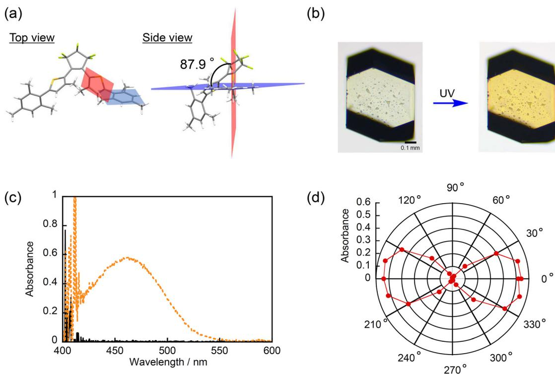
Fig. 5 (a) Molecular structure of **6o** in crystal **6o- $\alpha$**  determined by X-ray crystallographic analysis, (b) optical microphotographs of crystal **6o- $\alpha$**  before and after UV irradiation, (c) absorption spectra of crystal **6o- $\alpha$**  before and after UV irradiation, and (d) polar plots of the polarized absorption spectra of crystal **6o- $\alpha$**  at 462 nm on the (001) face.
