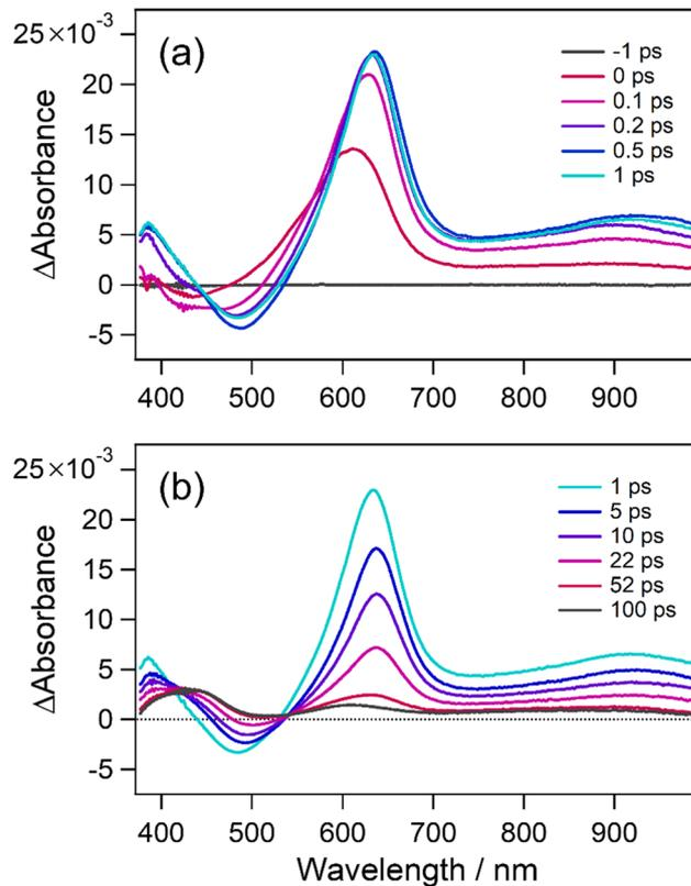
Fig. 2 Transient absorption spectra of **6o** in *n*-hexane solution ( $1.0 \times 10^{-3} \text{ mol L}^{-1}$ ) in (a) early and (b) late time regions. The sample was excited with a femtosecond laser pulse at 350 nm. The excitation power was 120 nJ per pulse.
