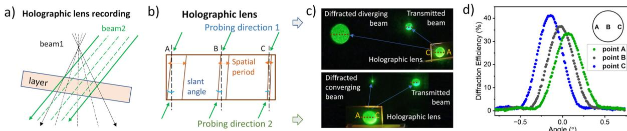
**Fig. 6** (a) Recording of the holographic lens by overlapping a divergent laser beam (beam1) and a collimated laser beam (beam2). (b) Schematic representation of the spatial period and the slant angle across the holographic lens. (c) Photographs of the diffraction produced by the holographic lens when probing from the same direction as recording (probing direction 1) and the opposite one (probing direction 2), respectively. (d) Diffraction efficiency along the horizontal diameter.
