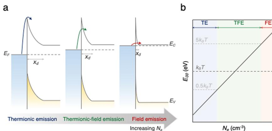
**Fig. 2** (a) Schematic representation of the carrier transport at the metal–semiconductor interface as doping concentration increases. (b)  $E_{00}$  as a function of doping density, illustrating the three charge injection modes: thermionic emission (TE) when  $E_{00} \leq 0.5kT$ , thermionic-field emission (TFE) when  $0.5kT < E_{00} < 5kT$ , and field emission (FE) when  $5kT \leq E_{00}$ .
