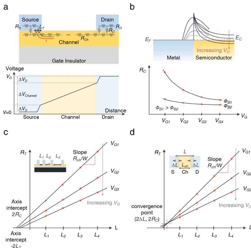
Fig. 3 (a) Schematic representation of a device illustrating the resistor network  $R_T = R_{ch} + 2R_C$ , along with a voltage profile indicating the voltage drop across the drain–channel–source region. (b) Energy band diagram showing the barrier decreasing as  $V_G$  increases, with a plot demonstrating the  $V_G$  dependence of  $R_C$  for high  $V_G$  and low  $\Phi_B$ . (c), (d) Schematic graphs for a transmission line method (TLM) of  $R_T$  as a function of  $L$ .
