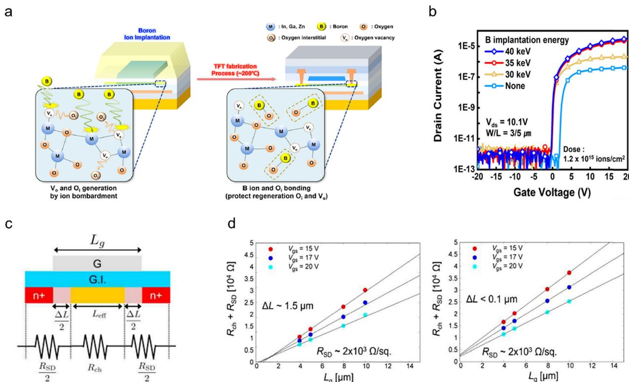
Fig. 6 (a) Schematic illustration of the reaction of B ions implanted in the IGZO surface. (b) The  $I$ - $V$  characteristics at different B implantation energies. (c) Illustration of S/D series resistance  $R_{ch} + R_{SD}$  at the gate edges in TFTs. (d) Measurements of the S/D series resistances in  $Ne^+$  (left) or  $B^+$  (right) implanted TFTs as a function of gate length ( $L_g$ ) for  $V_G$  of 15, 17, and 20 V.
