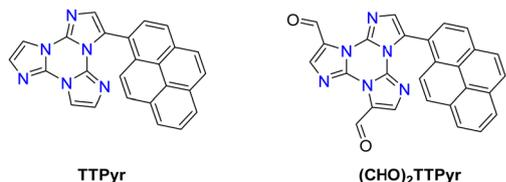
Scheme 19 Chemical structures of **TTPyr** and **(CHO)<sub>2</sub>TTPyr**.
