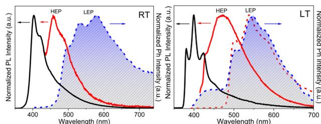
**Fig. 32** Normalized emission spectra of **TT-(C)-Cz** crystals at 298 K (left) and 77 K (right). PL (continuous line)  $\lambda_{\text{exc}} = 300$  nm (black) and  $\lambda_{\text{exc}} = 415$  nm (red), delayed spectra (dashed line)  $\lambda_{\text{exc}} = 385$  nm (298 K, delay 1 ms, window 5 ms; 90 K, blue: delay 0.5 ms, window 0.5 ms; red: delay 10 ms, window 20 ms).
