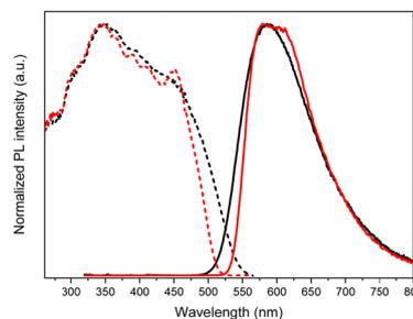
Fig. 45 Normalized excitation (dashed) and PL emission (continuous) spectra of crystalline powders of  $[\text{Cu}_2\text{I}_2(\text{TT-2Py})]_n$  at 298 K (black,  $\lambda_{\text{em}} = 588 \text{ nm}$ ;  $\lambda_{\text{exc}} = 300 \text{ nm}$ ) and 77 K (red,  $\lambda_{\text{em}} = 580 \text{ nm}$ ;  $\lambda_{\text{exc}} = 300 \text{ nm}$ ). Reproduced from ref. 130 under the terms of the Creative Commons CC BY license. Copyright 2023 by the authors. Licensee MDPI, Basel, Switzerland.
