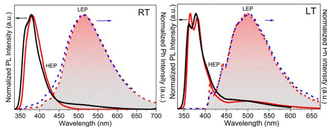
**Fig. 31** **TT-(C)-Cz** normalized emission spectra ( $\lambda_{\text{exc}} = 300$  nm). PL of DCM solutions ( $2 \times 10^{-6}$  M, red continuous) at 298 K (left) and 77 K (right). PL of PMMA films (0.5 wt%, at 298 K, left, and 90 K, right) in vacuum (black) and delayed spectra (blue dashed, delay 0.2 ms, window 0.5 ms; red dashed, delay 50 ms, window 10 ms) at 95 K.
