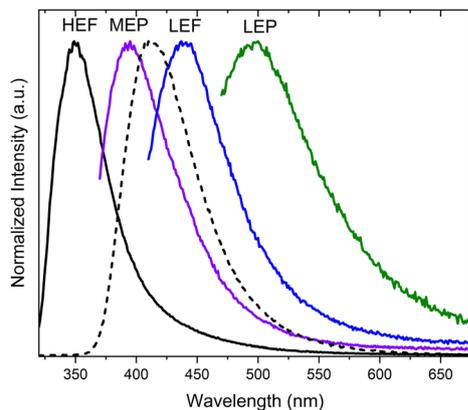
Fig. 37 Photophysical properties of **TT-2Py** in PMMA (**TT-2Py**/PMMA 10% wt) before (solid lines) and after (dashed line) HCl exposure. PL emission spectra  $\lambda_{\text{exc}} = 300$  nm (black lines),  $\lambda_{\text{exc}} = 350$  nm (violet),  $\lambda_{\text{exc}} = 390$  nm (blue), and  $\lambda_{\text{exc}} = 450$  nm (green).
