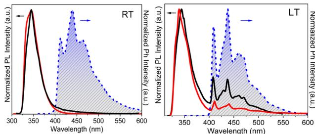
**Fig. 28** **TT-(N)-Cz** normalized emission spectra ( $\lambda_{\text{exc}} = 300$  nm). PL of DCM solutions ( $10^{-6}$  M, red) at 298 K (left) and 77 K (right) in air. PL of PMMA films (0.5 wt%) in vacuum (black) and delayed spectra (blue dashed; delay 200  $\mu\text{s}$ , window 500  $\mu\text{s}$  at 298 K (left); delay 5 ms, window 10 ms at 95 K (right)).
