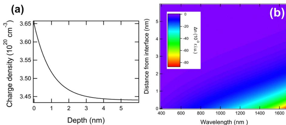
Fig. 7 (a) Charge profile in the AZO film as a function of the distance from the AZO/BTO interface as extracted from the modelling of the ellipsometric data. (b) Variations of the refractive index  $\Delta n$  as a function of wavelength and distance from the AZO/BTO interface.
