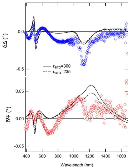
Fig. 6 Measured and modelled differentials  $\delta\Delta$  and  $\delta\Psi$  of the ellipsometric angles with a +0.2 V bias applied. The solid (dashed) lines represent the calculated  $\delta$ -spectra considering a value of  $\epsilon_{\text{BTO}} = 235$  ( $\epsilon_{\text{BTO}} = 300$ ) where both the Pockels effect in BTO and the charge accumulation at the AZO/BTO and NSTO/BTO interfaces are taken into account.
