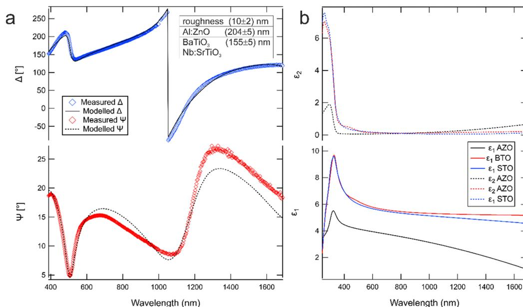
Fig. 4 (a) Measured and modelled ellipsometric angles  $\Delta$  and  $\Psi$  for the capacitor without the bias. (b) Real and imaginary parts of the dielectric function of every layer of the capacitor as extracted from ellipsometry.
