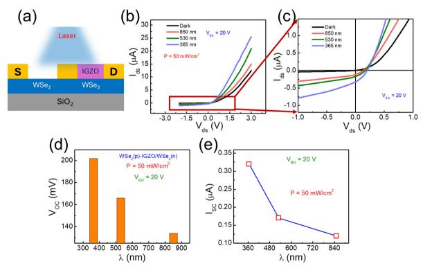
Fig. 4 (a) Schematic of the WSe<sub>2</sub> and IGZO/WSe<sub>2</sub> devices under laser source. (b) Gate-dependent output characteristics ( $I_{ds}$ – $V_{ds}$ ) of the device under different wavelengths at  $V_{BG}$  = 20 V. (c) Enlarged view of  $I_{ds}$ – $V_{ds}$  curves of the device. (d) and (e) Variation in the  $V_{OC}$  and  $I_{SC}$  of the device at  $V_{BG}$  = 20 V with the wavelength of illumination source at P = 50 mW cm<sup>-2</sup>.
