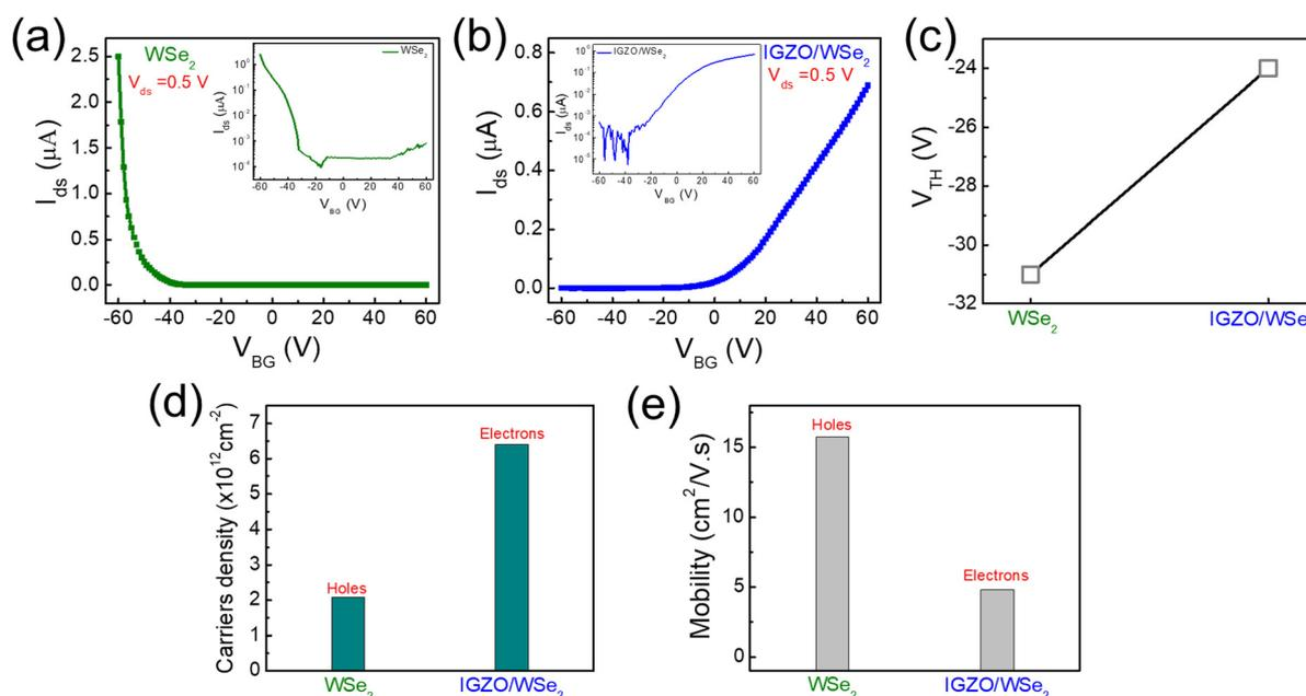
Fig. 2 (a) and (b) Transfer curves ( $I_{ds}$ - $V_{BG}$ ) with logarithmic insets. (c) Threshold voltage, (d) carrier concentration, and (e) field-effect mobility of electrons and holes of WSe<sub>2</sub> and IGZO/WSe<sub>2</sub>.
