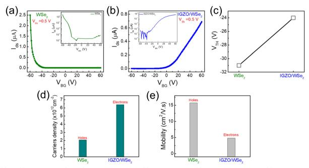
Fig. 2 (a) and (b) Transfer curves ( $I_{ds}$ - $V_{BG}$ ) with logarithmic insets. (c) Threshold voltage, (d) carrier concentration, and (e) field-effect mobility of electrons and holes of WSe<sub>2</sub> and IGZO/WSe<sub>2</sub>.
