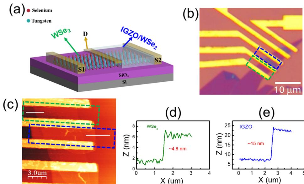
Fig. 1 (a) Schematic of the fabricated WSe<sub>2</sub> and IGZO/WSe<sub>2</sub> FETs. (b) Optical microscopy image of the WSe<sub>2</sub> flake with IGZO deposition on the Si/SiO<sub>2</sub> substrate. (c) AFM image of the IGZO and WSe<sub>2</sub> thin film. (d) Height profile of the WSe<sub>2</sub> flake and (e) IGZO.
