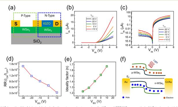
Fig. 3 (a) Schematic of the fabricated device indicating p-type and n-type regions for WSe<sub>2</sub> and IGZO/WSe<sub>2</sub>, respectively. (b) Gate dependent I-V curves on a linear scale. (c) Output characteristics (I<sub>ds</sub>-V<sub>ds</sub>) of the homo-PN diode (p-WSe<sub>2</sub>/n-IGZO·WSe<sub>2</sub>) on a logarithmic scale. (d) Rectification ratio (RR) of the homo-PN diode. (e) Ideality factor of the homo-PN diode. (f) Energy band diagram of the WSe2 p-n homojunction under light.
