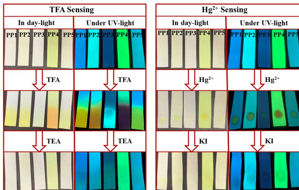
Fig. 16 Paper strips of PP1–PP5 employed to sense TFA and Hg<sup>2+</sup> ions in daylight and under UV light (365 nm).
