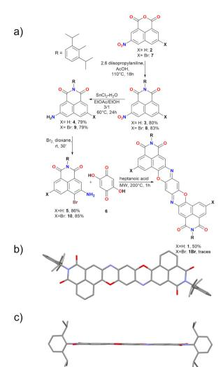
Scheme 1 (a) Synthesis of derivative 1, R = diisopropylphenyl; (b) top view and (c) side view of crystal structure of 1. Crystals obtained from slow diffusion of hexane in CHCl3. Space group: P21/n. Atom colours: O: red, N: blue, C: grey. Hydrogens omitted for clarity. CCDC 2383220.†
