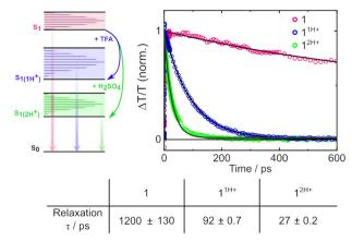
Fig. 3 Energy level diagram for 1 under neutral conditions, in TFA and in TFA + 0.2 M H<sub>2</sub>SO<sub>4</sub> where vertical arrows depict the probed transition of relaxation from  $S_1$  to  $S_0$ , alongside the dynamics of this process in each molecule and the associated lifetimes from global fitting to TA spectra in Fig. 2
