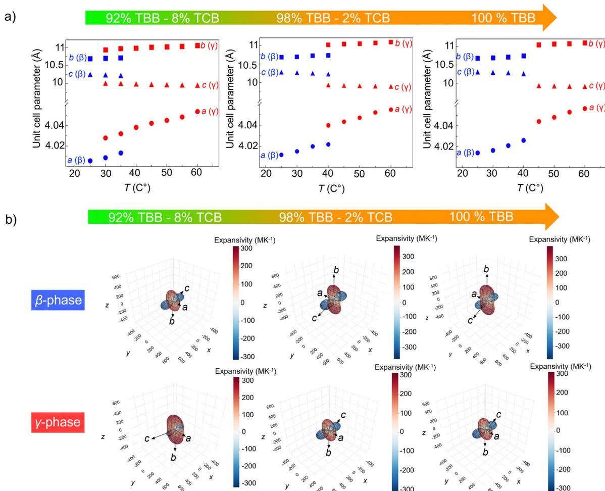
Fig. 3 (a) Temperature dependence of the unit-cell parameters of the low temperature  $\beta$ - and high temperature  $\gamma$ -phase for the molecular alloys containing 92, 98 and 100 wt% of TBB. (b) Thermal expansivity indicatrix of low temperature  $\beta$ - and high temperature  $\gamma$ -phase for the molecular alloys containing 92, 98 and 100 wt% of TBB.
