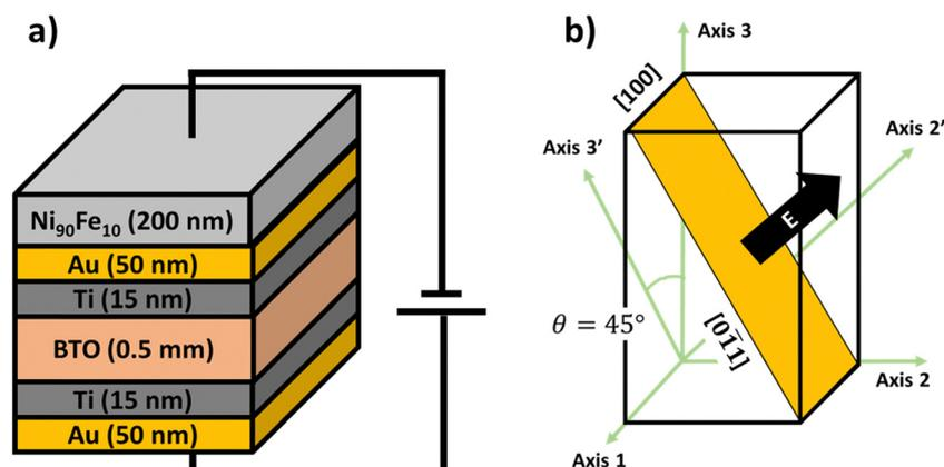
Fig. 1 (a) Schematic drawing of the studied heterostructure showing the applied electric voltage. (b) BTO(011) surface (yellow) showing the IP directions,  $[100]$  and  $[0\bar{1}1]$ , and the electric field applied in the OOP direction for the BTO(011) orientation studied in this work. The green axes represent the coordinate axes for the piezoelectric matrix. Axes 2' and 3' are obtained after a rotation of  $\theta = 45^\circ$  around axis 1.
