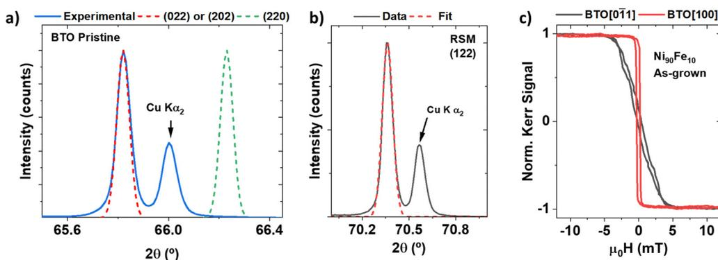
Fig. 2 (a)  $\theta$ - $2\theta$  XRD measurements of pristine BTO(011) (blue line) compared with possible surface orientations (red and green dashed lines). (b) RSM measurement (black line) of the (122) reflection and corresponding fit (red dashed line). (c) MOKE hysteresis loops of as-grown  $Ni_{90}Fe_{10}$  layer along IP hard and easy directions, corresponding to in-plane BTO  $[0\bar{1}1]$  (black line) and  $[100]$  directions (red line), respectively.
