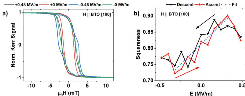
Fig. 4 (a) IP MOKE hysteresis loops for  $\text{Ni}_{90}\text{Fe}_{10}$  taken along the BTO [100] direction at several polings. (b) Squareness ( $M_r/M_s$ ) represented as a function of poling. Descent (black down triangles) and ascent (red up triangles) electric paths are shown differently for clarity. The linear fit of  $\frac{\Delta(M_r/M_s)}{\Delta E}$  is used to obtain  $\alpha_E$  according to eqn (6) of the main text.
