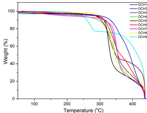
Fig. 6 TGA thermograms of **DCH<sub>1-9</sub>** determined at a heating rate of  $10\text{ }^\circ\text{C min}^{-1}$  under a nitrogen atmosphere.
