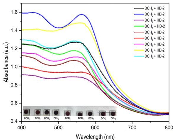
Fig. 5 UV-vis absorption spectra of **DCH<sub>1-9</sub>** + **HD-2** adsorbed on the **TiO<sub>2</sub>** surface.
