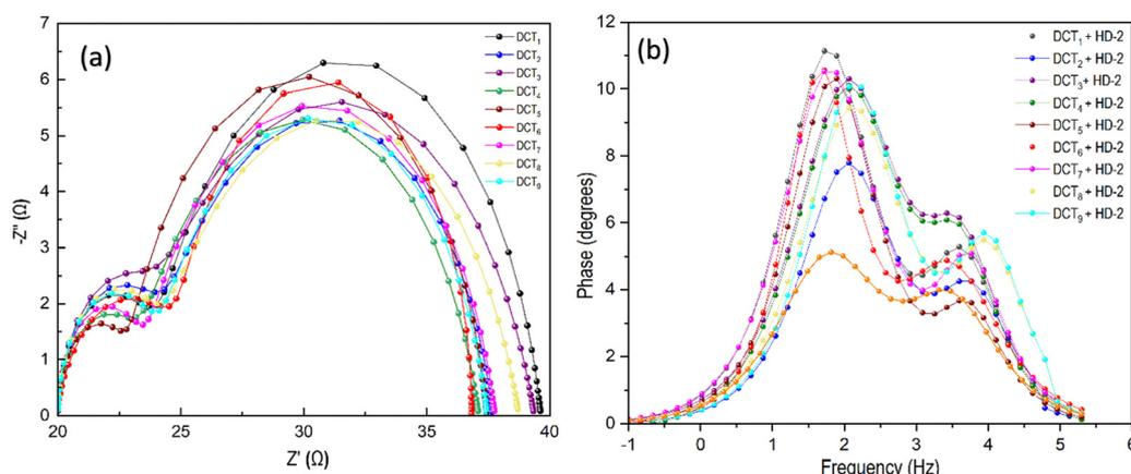
Fig. 11 EIS spectra of devices co-sensitized with **HD-2** using **DCH**<sub>1-9</sub>: (a) Nyquist plots, (b) Bode phase plots.
