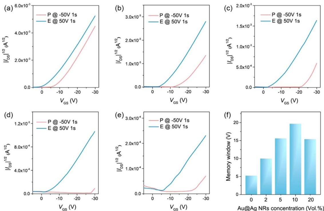
Fig. 3 Memory characteristics of (a) PVPy, (b) NRs-2, (c) NRs-5, (d) NRs-10 and (e) NRs-20 memory devices in programmed and erased states. (f) Comparison of memory windows with different concentrations of Au@Ag NRs. Reprinted (adapted) with permission from ref. 77. Copyright 2022 American Chemical Society.
