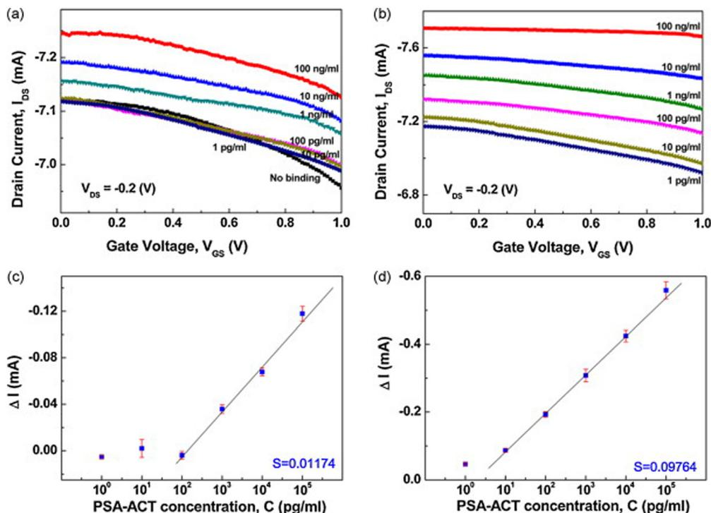
Fig. 7  $I$ - $V$  curve of the OECT based immunosensor (a) without AuNP, and (b) with AuNP. (c) and (d) calibration curve without and with AuNPs respectively. Reprinted from ref. 94 with permission from Elsevier.
