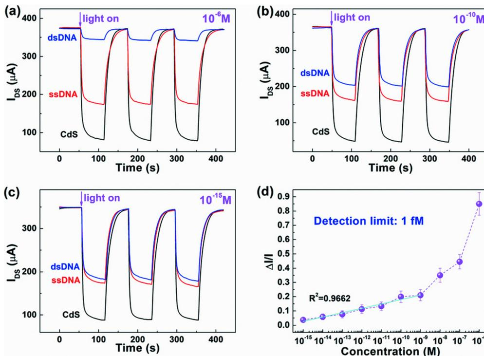
Fig. 9 (a)–(c) represent channel current versus time for  $1 \times 10^{-6}$  M,  $1 \times 10^{-10}$  M and  $1 \times 10^{-15}$  M respectively, and (d)  $\Delta I/I$  versus concentration of target ssDNA,  $R$  being the linear regression equation parameter. Reproduced with permission from ref. 95 © 2018 WILEY-VCH Verlag GmbH & Co. KGaA, Weinheim.
