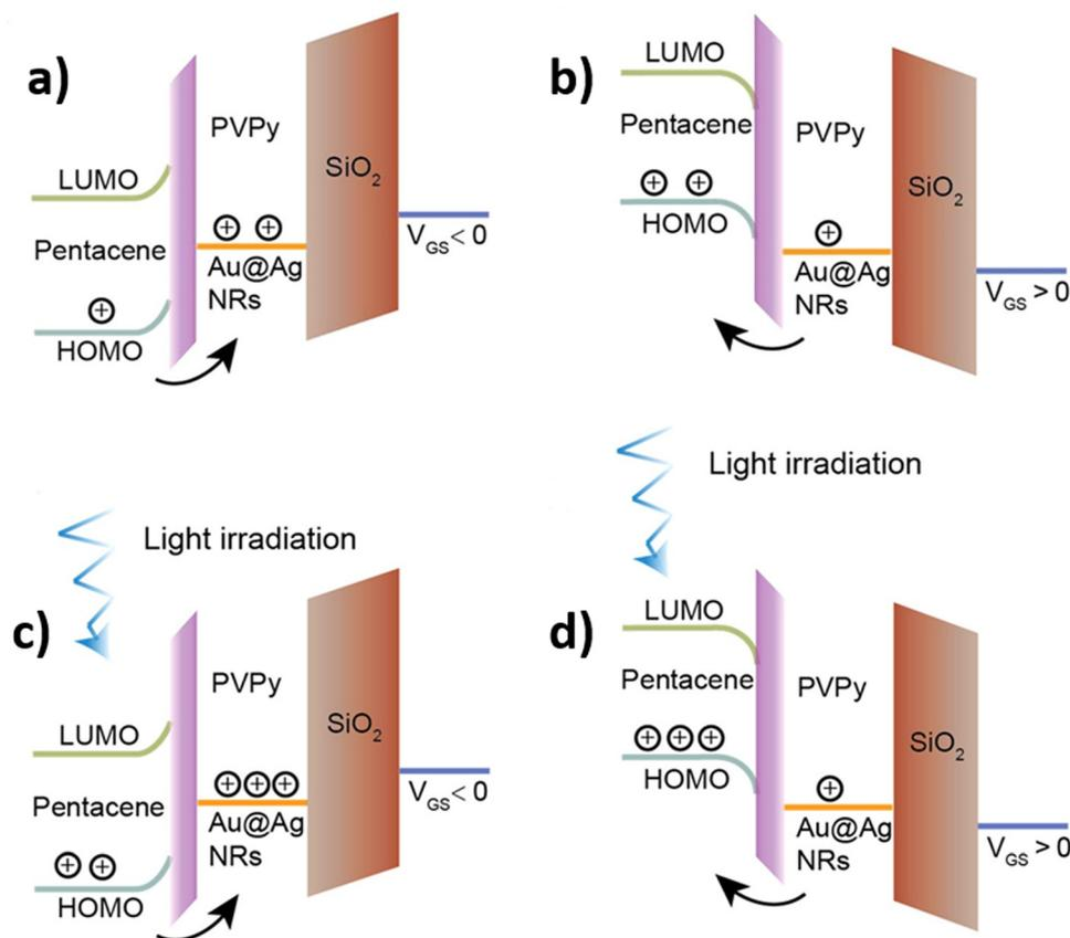
Fig. 4 Energy band diagram of OFET optical memory device (a) In the dark while programming, (b) In the dark while erasing, (c) while programming under light irradiation and (d) while erasing under light irradiation. Reprinted (adapted) with permission from ref. 77. Copyright 2022 American Chemical Society.
