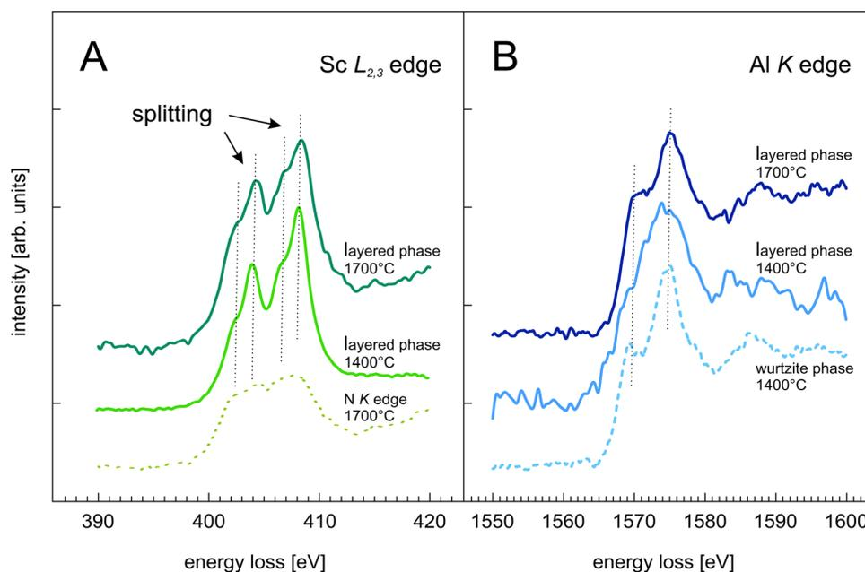
**Fig. 3** EELS spectra of (A) Sc  $L_{2,3}$  and (B) Al K edge. Both spectral lines of Sc  $L_{2,3}$  edge (A) are split by nearly 2 eV indicating octahedral coordination for Sc. Sc  $L_{2,3}$  spectra were superimposed by the broad N K edge, given separately for the 1700 °C spectra at the bottom (dashed). Independent of the annealing temperature, Al K edge spectra (B) of the layered phases are identical to those of AlN of the wurtzite structure (dashed), indicating tetrahedral coordination.
