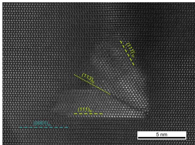
Fig. 5 STEM-HAADF image of a  $\text{Sc}_2\text{O}_3$  nanocrystal at the (Al,Sc)N grain boundary showing a twin-like intergrowth along the common  $(113)_{\text{bi}}$  plane. The crystal orientation refers to the  $[2\bar{1}\bar{1}0]_{\text{w}}$  zone axis of (Al,Sc)N and  $[1\bar{1}0]_{\text{bi}}$  of  $\text{Sc}_2\text{O}_3$ .
