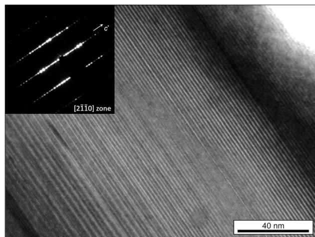
Fig. 1 TEM bright-field image showing bright planes expanding laterally straight up to grain boundaries. The corresponding SAED pattern (inset) along the [2 $\bar{1}$ 10] zone axis agrees well with a hexagonal lattice but shows quite complex superstructure reflections along the *c*\*-direction.
