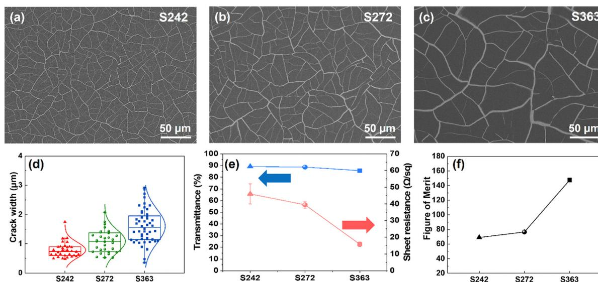
Fig. 4 FE-SEM images of the micro-mesh grid obtained using the silica solution concentrations of (a) 0.242 (S242), (b) 0.272 (S272), and (c) 0.363  $\text{g mL}^{-1}$  (S363). (d) Distribution of crack widths, (e) transmittance and sheet resistance, and (f) FoM of the transparent electrodes as a function of the silica solution concentration.
