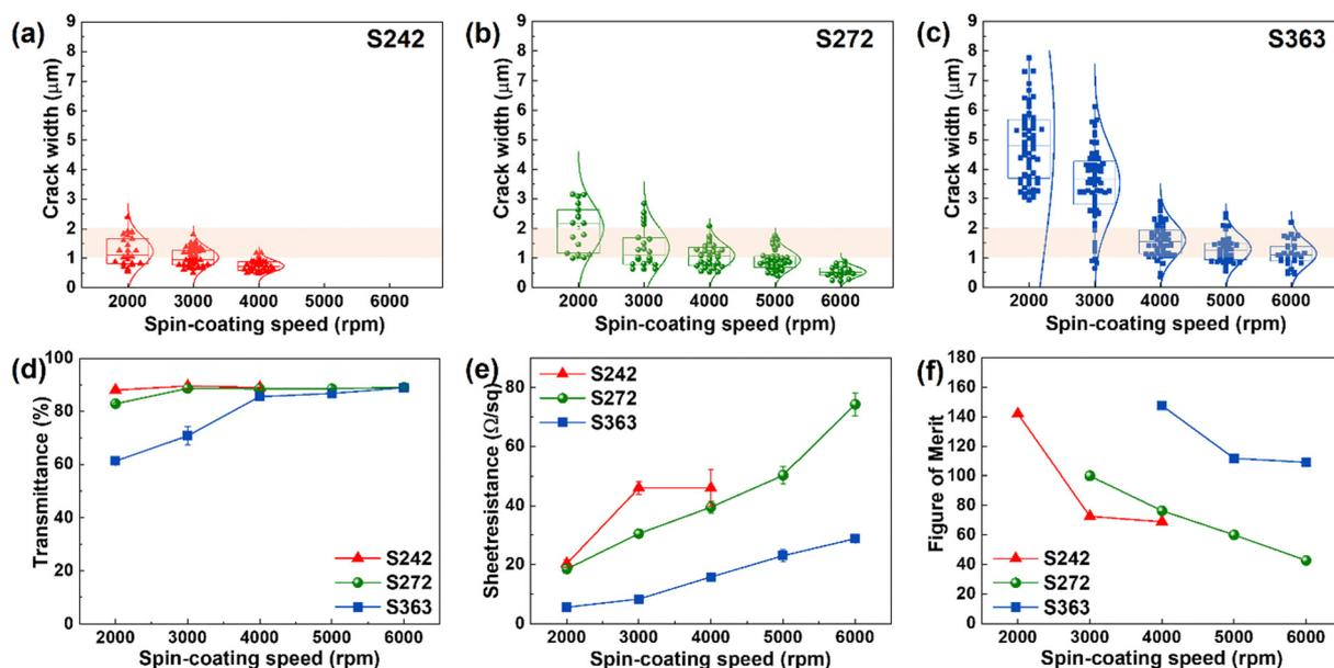
Fig. 5 Distributions of the crack width values of (a) S242 (0.242 g mL<sup>-1</sup>), (b) S272 (0.272 g mL<sup>-1</sup>), and (c) S363 (0.363 g mL<sup>-1</sup>) samples as a function of spin-coating speed. (d) Transmittance, (e) sheet resistance, and (f) FoM of the S242, S272, and S363 samples as a function of spin-coating speed.
