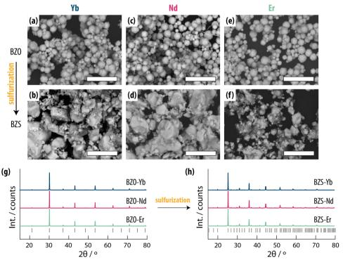
Fig. 3 SEM images of BZO-Yb (a), BZS-Yb (b), BZO-Nd (c), BZS-Nd (d), BZO-Er (e) and BZS-Er (f). Scale bars are 10 μm. XRD patterns of BZO-Ln series (g) and of BZS-Ln series (h). Vertical grey lines in (g) and (h), respectively indicate the position of the Bragg reflections for BaZrO<sub>3</sub> and BaZrS<sub>3</sub>.
