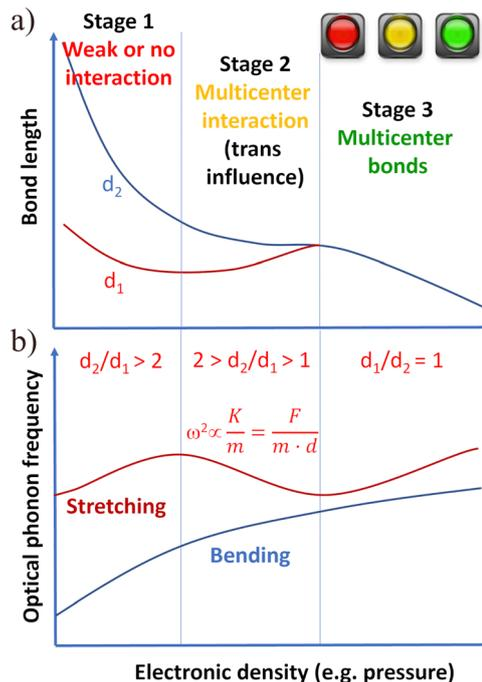
Fig. 2 General behavior of the (a) bond lengths and (b) optical phonon frequencies of a material with a primary and a secondary bond, which are linked by a *trans* influence, and therefore lead to the multicenter bond formation upon the increase of the electronic density; *e.g.* upon reduction, increase of pressure, or chemical substitution of an element by a heavier analog.
