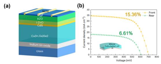
Fig. 14 (a) Device structure of a bifacial CIGS solar cell fabricated on a glass substrate. (b) J-V curves of flexible bifacial CIGS device under front and rear illumination, with a simplified scheme of the device architecture. (Reproduced and adapted from ref. 142 with permission from Springer Nature, Copyright 2022).
