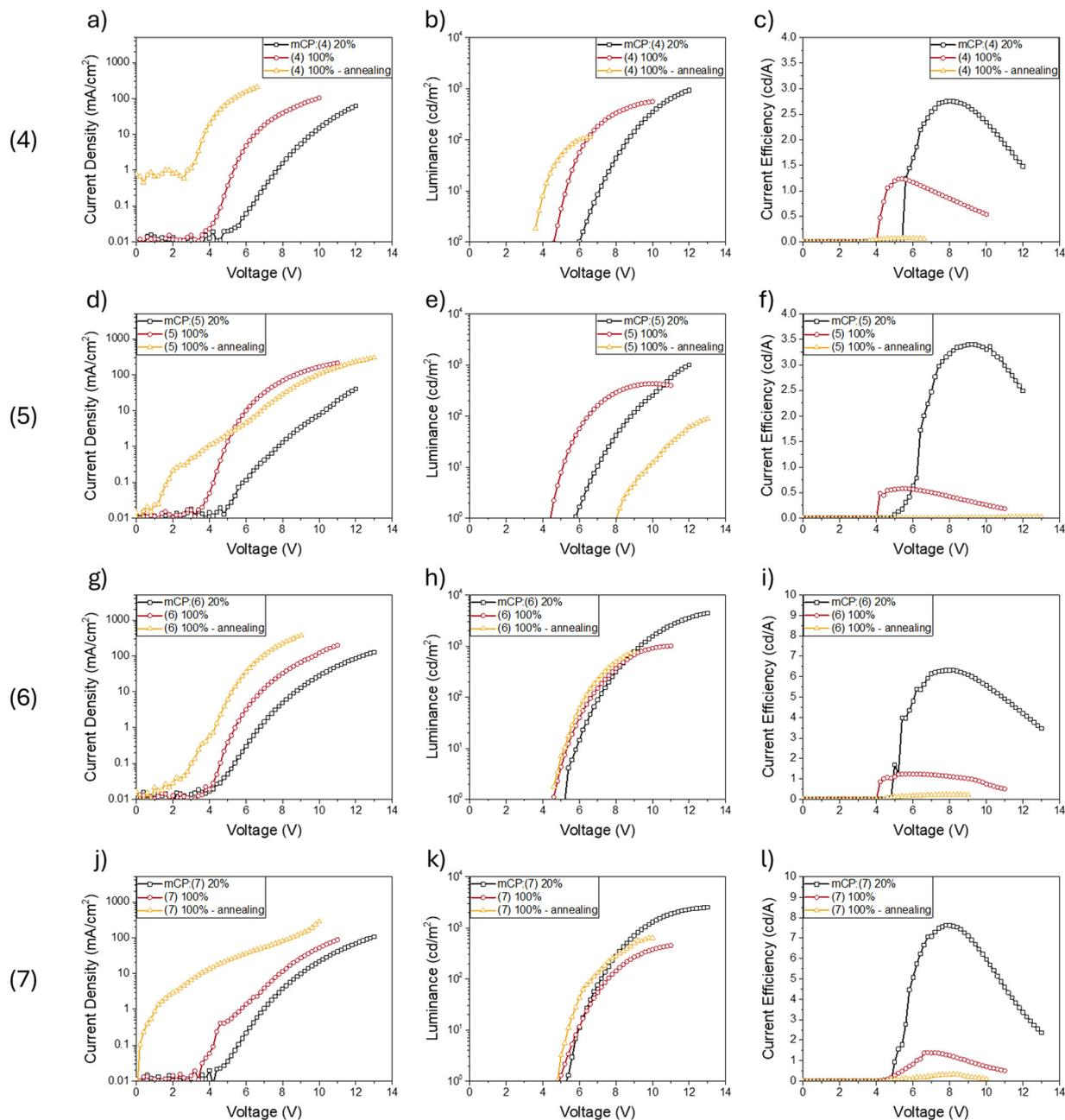
Fig. 6 Electroluminescent characteristics of OLEDs using **4**, **5**, **6** and **7** as the active layer, dispersed in an appropriate matrix (mCP) and in neat film (with or without annealing). Voltage vs. current density, voltage vs. luminance and voltage vs. efficiency for molecules **4** (a)–(c), **5** (d)–(f), **6** (g)–(i) and **7** (j)–(l).
