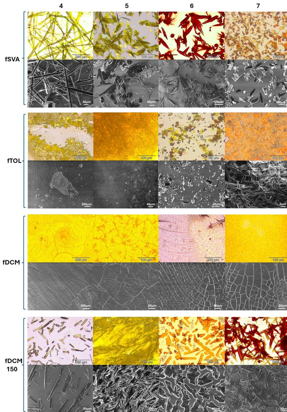
Fig. 3 Surface morphology of samples 4–7 prepared using the different processing methods (fDCM, fTOL, fSVA, and fDCM150). Top panels (colour images) show optical microscopy photographs. Bottom panels (black and white images) display the corresponding scanning electron microscopy (SEM) images. The images revealing microscale surface features and morphological variations induced by the preparation methods. Scale bars are included in all optical and SEM images.
