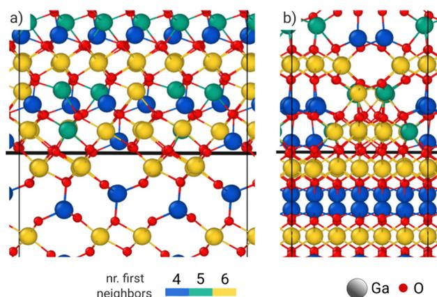
Fig. 6 Front (a) and side (b) views of the  $\kappa$ -Ga<sub>2</sub>O<sub>3</sub>/ $\beta$ -Ga<sub>2</sub>O<sub>3</sub> interface.  $\beta$ -Ga<sub>2</sub>O<sub>3</sub> interlayer is fully strained on the  $\alpha$ -Al<sub>2</sub>O<sub>3</sub> substrate. The black line marks the plane of O atoms shared by both film and substrate.
