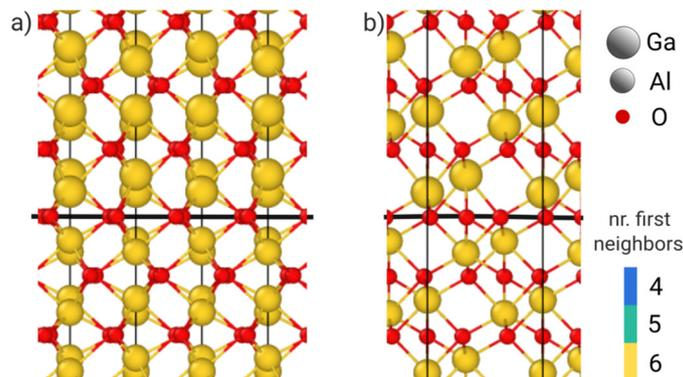
Fig. 3 Front (a) and side (b) view of the  $\alpha$ -Ga<sub>2</sub>O<sub>3</sub>/ $\alpha$ -Al<sub>2</sub>O<sub>3</sub> interface. The black line marks the plane of O atoms shared by both film and substrate.
