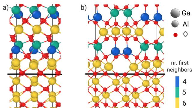
Fig. 5 Front (a) and side (b) view of the  $\kappa$ -Ga<sub>2</sub>O<sub>3</sub>/ $\alpha$ -Al<sub>2</sub>O<sub>3</sub> interface. The black line marks the plane of O atoms shared by both the film and the substrate.
