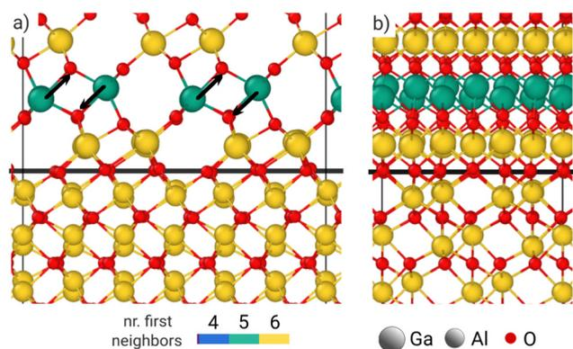
Fig. 4 Front (a) and side (b) view of the  $\beta$ -Ga<sub>2</sub>O<sub>3</sub>/ $\alpha$ -Al<sub>2</sub>O<sub>3</sub> interface. The black line marks the plane of O atoms shared by both film and substrate.
