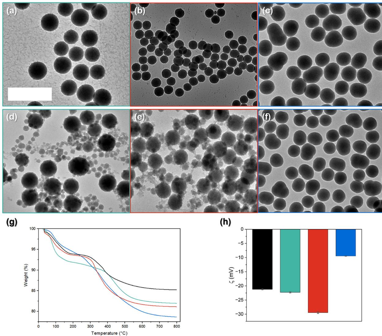
Fig. 2 Micrographs of particles prepared using TEOS and either (a)–(c) 10 or (d)–(f) 30 mol% of (a) and (d) CPTES, (b) and (e) MPTES, or (c) and (f) APTES. Scale bars represent 500 nm. (g) TGA and (h) measured Zeta potential of the four systems: silica (black), and the hybrids CPTES (green), MPTES (red), and APTES (blue) prepared with 70/30 mol%.
