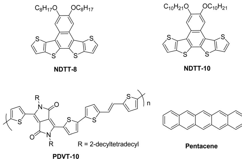
**Fig. 71** Molecular structures of the organic semiconductors **NDTT-8**, **NDTT-10**, **PDVT-10** and pentacene.
