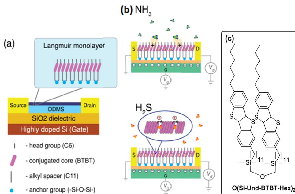
Fig. 10 (a) LS OFET device architecture. (b) Suggested mechanisms of  $\text{NH}_3$  and  $\text{H}_2\text{S}$  (reproduced with permission from ref. 84. Copyright 2018, ACS). (c) Chemical structure of the organosilicon dimer  $\text{O}(\text{Si-Und-BTBT-Hex})_2$  in the closed conformation.
