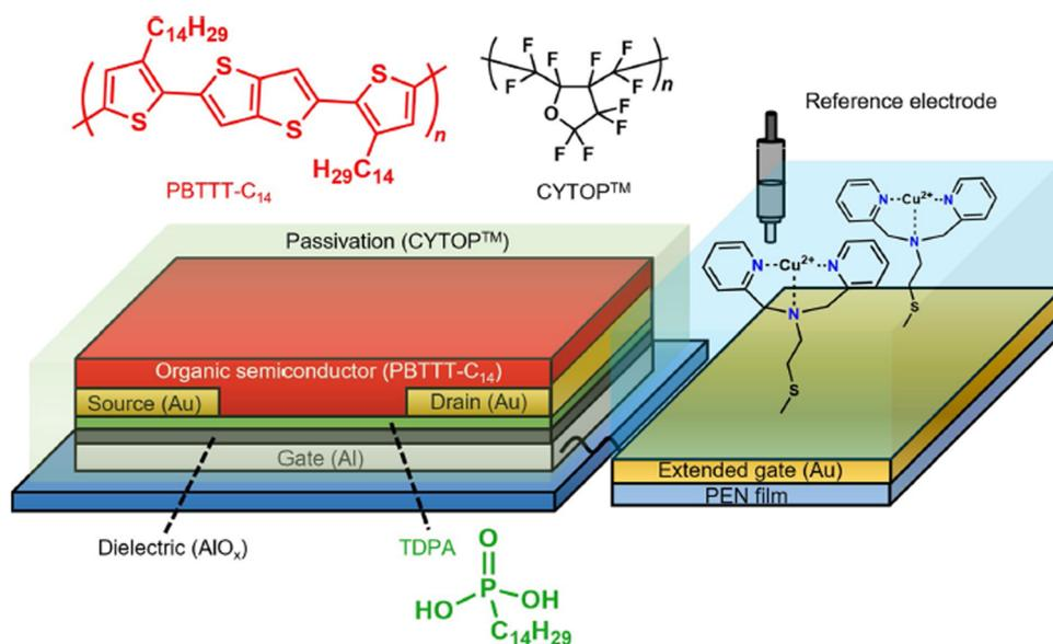
Fig. 39 Schematic of the EG-OFET structure for CS detection. The extended-gate electrode portion was modified with the  $\text{Cu}^{2+}$ -dpa complex (reproduced with permission from ref. 155. Copyright 2022, Springer Nature).
