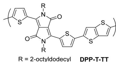
Fig. 21 Chemical structure of the OSC polymer **DPP-T-TT**.
