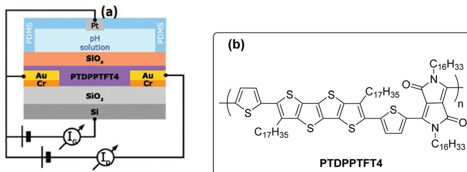
Fig. 37 (a) A pH sensor based on the BGBC dual-gate OFET and SiO<sub>x</sub> as the active sensing layer (reproduced with permission from ref. 134. Copyright 2019, WILEY), (b) chemical structure of PTDPPTFT4 used as a semiconductor.
