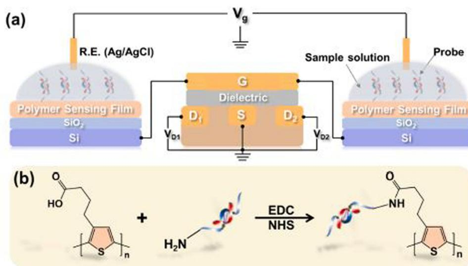
**Fig. 75** (a) Schematic of the remote dual-gated FET sensing system: the two remote gates are connected in parallel to the gates of the commercial transistor. (b) Functionalization of the PT-COOH film with probe VEap/CS to form the PT-VEap sensing surface on the remote gates using EDC/NHS chemistry. (Reproduced with permission from ref. 249. Copyright 2025, Elsevier.)
