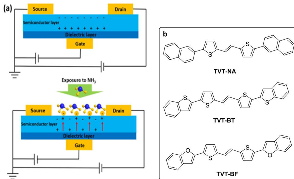
Fig. 18 (a) Schematic representation of the  $\text{NH}_3$  gas sensing mechanism (reproduced with permission from ref. 93. Copyright 2022, Elsevier); (b) molecular structures of thienylene–vinylene–thienylene (TVT) derivatives.
