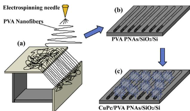
Fig. 5 Illustrations of CuPc growth on well-ordered PVA parallel nanofiber arrays (PNAs). (a) PVA PNAs receiving board. (b) PVA PNAs were transferred to SiO<sub>2</sub>/Si substrates. (c) CuPc was evaporated on PVA PNAs/SiO<sub>2</sub>/Si (reproduced with permission from ref. 68. Copyright 2021, Elsevier).
