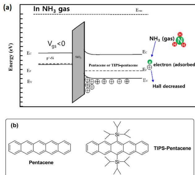
**Fig. 22** (a) Illustration of the mechanism of NH<sub>3</sub> gas sensing with OFET (reproduced with permission from ref. 97. Copyright 2022, Springer Nature). (b) Molecular structure of pentacene and TIPS-pentacene.
