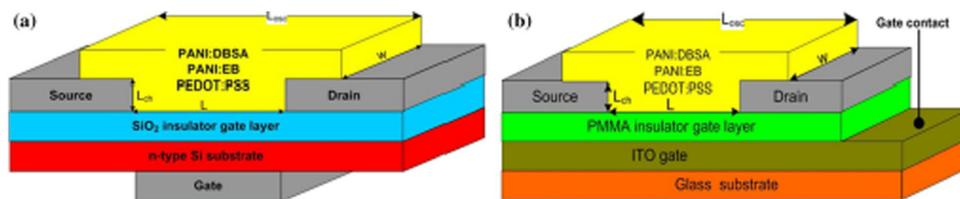
Fig. 23 Layout structures of the OFETs as ammonia sensors based on the (a) n-type Si gate with  $\text{SiO}_2$  insulator layer; (b) ITO gate with the PMMA insulator gate layer, where  $L_{\text{OSC}}$  = channel length,  $L$  = active channel thickness,  $L_{\text{ch}}$  = channel thickness, and  $w$  = channel width (reproduced with permission from ref. 98. Copyright 2019, Springer Nature).
