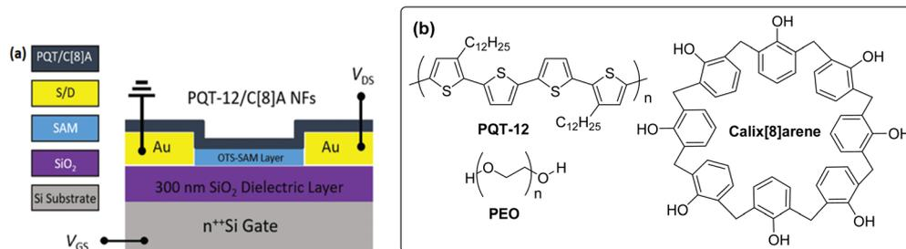
Fig. 42 (a) Schematic showing a **PQT-12/C[8]A** OFET device with an interdigitated S/D electrode (reproduced with permission from ref. 158. Copyright 2019, RSC), (b) the molecular structures of **PQT-12**, **C[8]A** and the poly(ethylene oxide) **PEO**.
