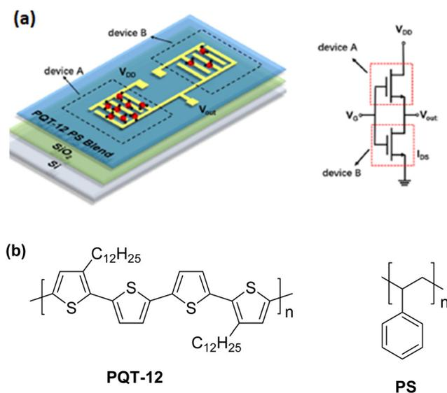
Fig. 13 (a) Structure and diagram of the OFET-based circuit (reproduced with permission from ref. 87. Copyright 2019, ACS) and (b) the chemical structure of PQT-12 and PS.
