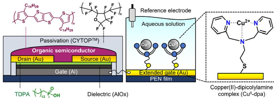
Fig. 40 Schematic of the extended-gate-type OFET for oxyanion detection. The extended-gate electrode was functionalized with the Cu<sup>II</sup>-dpa complex (reproduced with permission from ref. 156. Copyright 2022, ACS).
