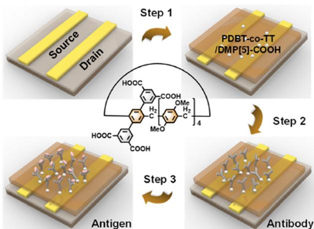
Fig. 66 The schematic representation of the OFET-based SiMoT platform. Step 1: the PDBT-co-TT/DMP[5]-COOH was spin-coated as the charge transport layer on the OTS-modified SiO<sub>2</sub>/Si substrate with the deposited Au source and drain electrodes; step 2: the antibodies were immobilized as sensitive probes for the determination of tumor biomarkers; step 3: the antibody-antigen recognition events (reproduced with permission from ref. 238. Copyright 2022, ACS).
