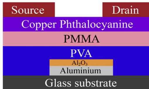
Fig. 45 Schematic diagram of the device fabricated using the top-contact bottom-gate configuration. The device contains the PMMA/PVA/Al<sub>2</sub>O<sub>3</sub> tri-layer gate dielectric material, aluminium as the gate electrode, CuPc as the organic semiconductor materials and copper as the source drain electrode material (reproduced with permission from ref. 178. Copyright 2013, Elsevier).
