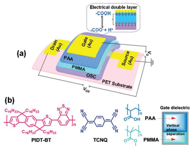
Fig. 30 (a) Structure of the flexible OFET device. (b) Molecular structures of **PIDT-BT**, **TCNQ**, **PAA**, and **PMMA** (inset is an illustration of the **PMMA/PAA** dielectric with a vertical phase separation structure) (reproduced with permission from ref. 121. Copyright 2018, WILEY).
