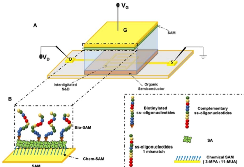
Fig. 72 (A) Three-dimensional schematic representation of the SiMoT device. (B) Schematic representation of the gate surface biofunctionalized with a biotinylated single-strand oligonucleotide. Chem-SAM is depicted by blue arrows, and the structures of the bio-SAM and target oligonucleotides (miR-182-5p) are sketched in the right panel (reproduced with permission from ref. 246. Copyright 2020, ACS).
