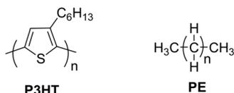
Fig. 44 Structures of poly(3-hexylthiophene-2,5-diyl) (P3HT) and polyethylene (PE).
