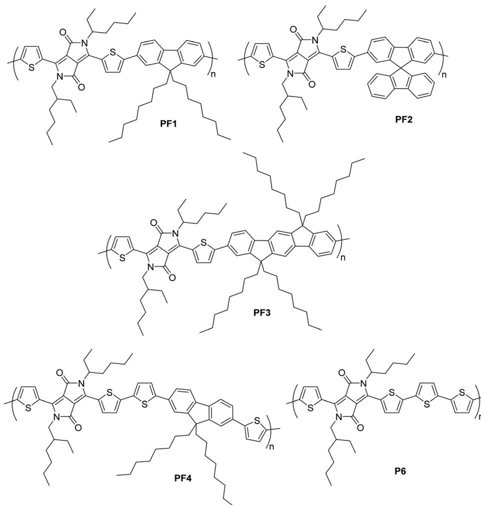
Fig. 15 Chemical structures of diketopyrrolopyrrole-fluorene and diketopyrrolopyrrole-bithiophene-based polymers.
