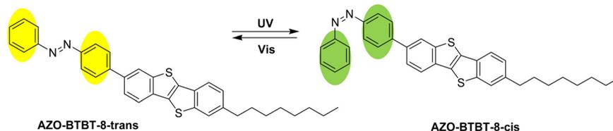
Fig. 49 Organic semiconductor AZO-BTBT-8 with photoisomerization property.
