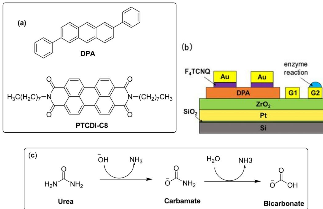
**Fig. 79** (a) Molecular structures of DPA and PTCDI-C8. (b) OFET device structure (reproduced with permission from ref. 252. Copyright 2025, ACS). (c) Proposed mechanism of urea hydrolysis under urease.
