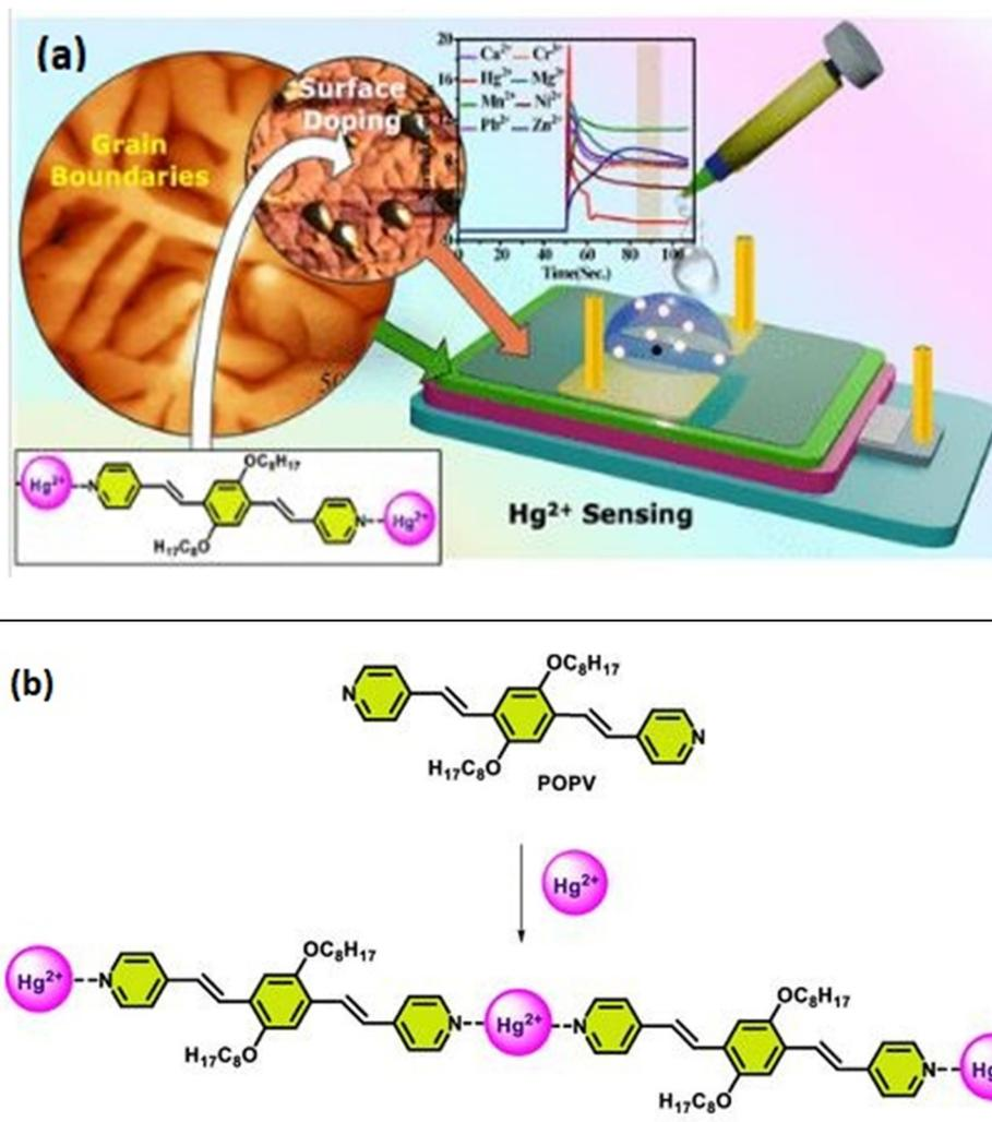
Fig. 77 (a) Schematic design showing the visual representation of the OFET highlighting the arrangement of the various layers involved. (b) Molecular structure of the mercury-sensing molecule POPV forming a coordination complex with mercury. (Reproduced with permission from ref. 250. Copyright 2025, ACS.)
