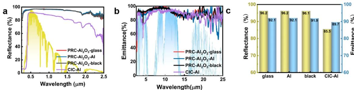
Fig. 4 Optical properties of the coatings. (a) UV-vis-NIR reflectance and (b) IR emissivity of PRC- $\text{Al}_2\text{O}_3$  and CIC presented against the AM1.5 solar spectrum (yellow) and the atmospheric transparency window (blue), respectively. (c) The corresponding reflectance and emissivity values in Fig. 4a and b.
