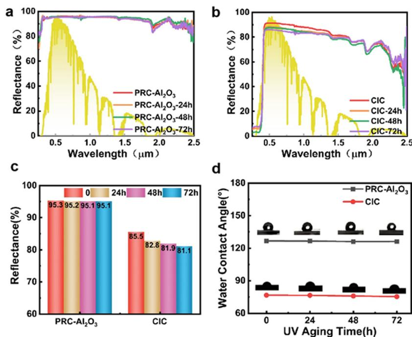
Fig. 6 The UV-vis-IR reflectance of (a) PRC- $\text{Al}_2\text{O}_3$  and (b) CIC before and after 72 h UV irradiation presented against the AM1.5 solar spectra (yellow), (c) calculated values of reflectance at different UV irradiation times. (d) Changes in the water contact angle before and after 72 h UV irradiation.
