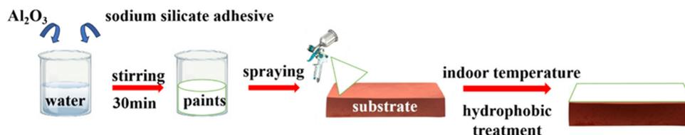
Fig. 1 Coating preparation process.
