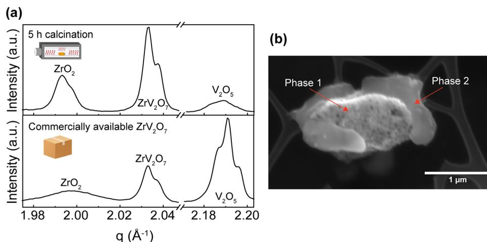
Fig. 2 (a) XRD of a solid-state 40' 5 h multi-phase material and commercially available  $\text{ZrV}_2\text{O}_7$  material. (b) SEM image (20 kV, SE) corresponds to the multi-phase solid-state 40' 5 h material.
