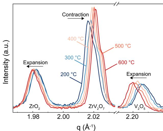
Fig. 8 *In situ* XRD characterisation of  $\text{ZrV}_2\text{O}_7$  sample synthesised via solid-state synthesis and calcined for 5 h at 700 °C. The peak corresponding to  $\text{ZrV}_2\text{O}_7$  shows unit cell contraction in the 200–500 °C range, while residual  $\text{ZrO}_2$  and  $\text{V}_2\text{O}_5$  phases display opposite unit cell expansion behaviour.
