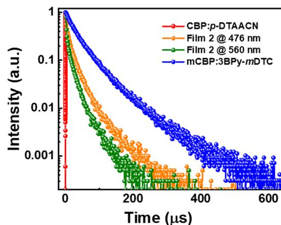
**Fig. 5** Transient photoluminescence decay curves of doped white film 2, observed at the PL emission peaks at 476 nm and 560 nm, overlay with CBP:*p*-DTAACN (emission wavelength 588 nm) and *m*CBP:7 wt% 3BPY-*m*DTC (emission wavelength 479 nm) films. The excitation wavelength of 340 nm was used for all the films.
