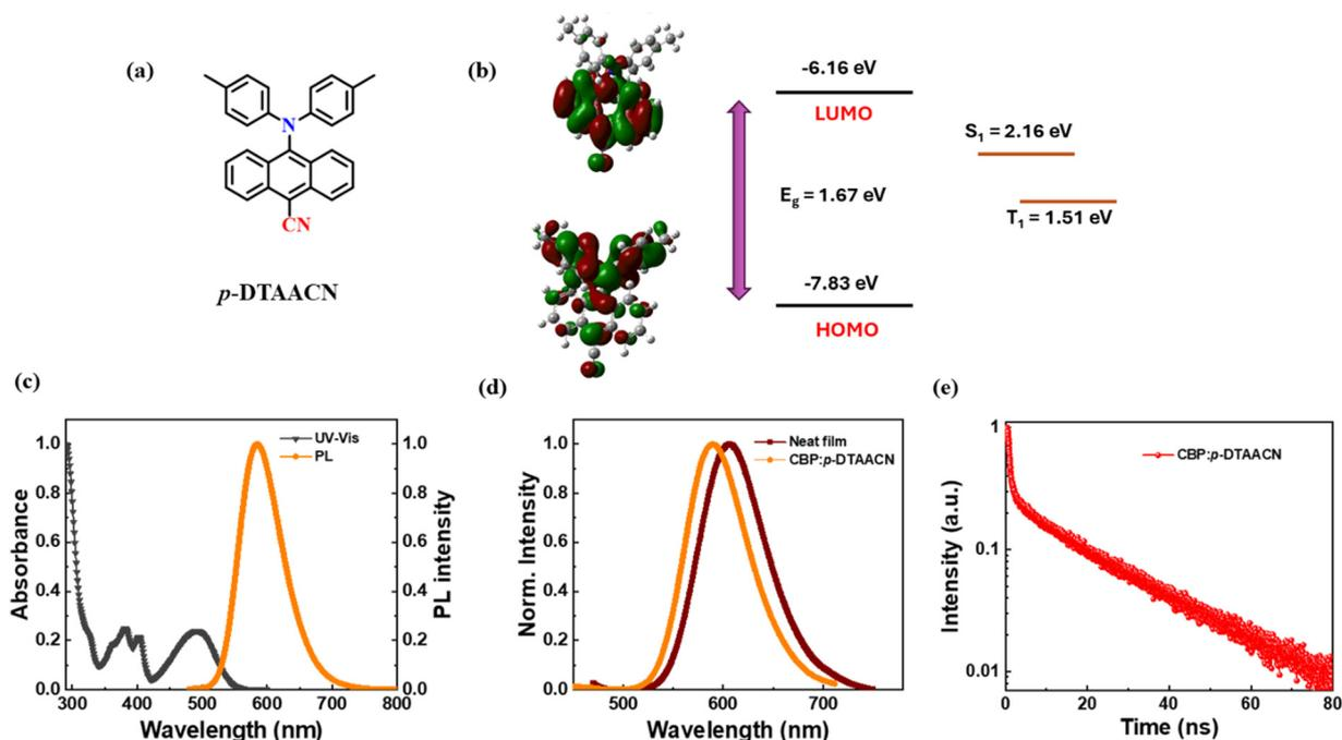
Fig. 1 (a) Molecular structure; (b) frontier orbital distribution and the calculated HOMO/LUMO energy levels and lowest singlet/triplet levels of *p*-DTAACN; (c) UV-vis absorption and fluorescence behaviour measured in  $10^{-5}$  M toluene; (d) photoluminescence spectra of the neat film and CBP doped film of *p*-DTAACN; and (e) the transient photoluminescence decay for the CBP:*p*-DTAACN doped film with excitation wavelength 340 nm and emission wavelength 588 nm.
