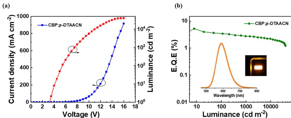
Fig. 2 (a) Dependence of current density–voltage–luminance ( $J$ – $V$ – $L$ ) curve and (b) plot of external quantum efficiency vs. luminance of  $p$ -DTAACN device. Insets: Electroluminescence spectra and the photo of the  $p$ -DTAACN device taken at 8 V.
