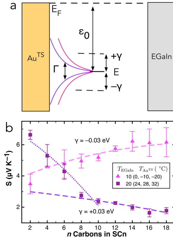
Fig. 6 A simplified schematic of how the applied electric field induces a Stark shift in the transport level  $E$  (a). Experimental values of  $S$  from Fig. 4 plotted with computed values of  $n$  using the range of  $\Gamma$  values from ref. 68 at  $\varepsilon = -0.96$  eV (dashed;  $-0.40$  eV dotted) with shifts of  $\pm 0.03$  eV (b).
