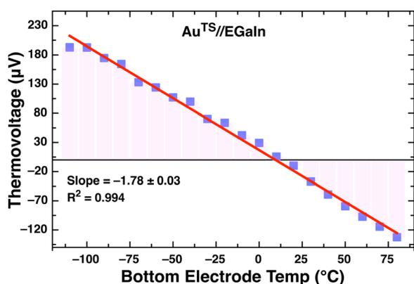
Fig. 2 Thermal voltage measurement of Au<sup>TS</sup>//EGaIn contact across the entire range of 80 to –120 °C.
