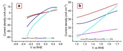
Fig. 12 LSV plots obtained with P1, P2, P3, and P4 MOFs for HER (a) and OER (b) at 5 mV s<sup>-1</sup> in 0.1 M KOH.
