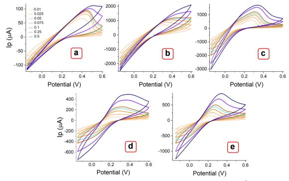
Fig. 8 CV curves of MOFs (a) E, (b) P1, (b) P2, (c) P3, and (d) P4, recorded at different scan rates from 0.01 to 0.5 V s<sup>-1</sup>.
