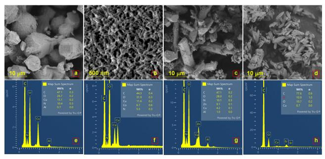
Fig. 2 SEM micrographs and corresponding EDS profiles of (a) and (b) E, (c) and (d) P1, (e) and (f) P2, (g) and (h) P3.
