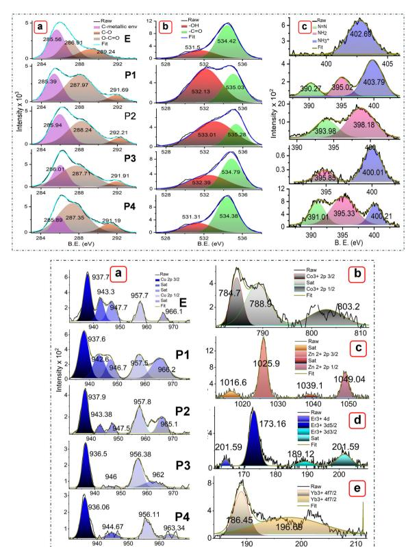
Fig. 5 (A) XPS spectra of (a) C1s, (b) O1s, and (c) N1s, in MOFs E, P1, P2, P3, and P4. (B) XPS spectra of (a) Cu in MOFs E, P1, P2, P3, and P4. (b) Co in P1, and (c) Zn in P2, (d) Er in P3, and (e) Yb in P4.
