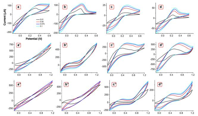
Fig. 10 Comparison of the electrochemical behavior of MOFs P1, P2, P3 and P4 using as synthesized (a)-(d), thermally treated 280 °C (a'-d'), and thermally treated 580 °C (a'-d') materials, respectively
