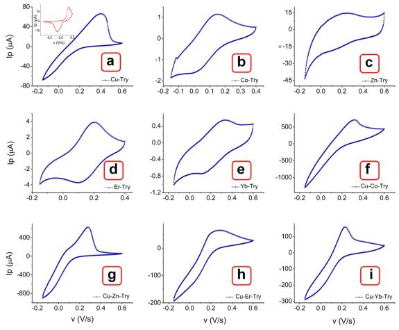
Fig. 11 Comparison of the voltammograms of single metal MOFs (a) – (e) with the multi centered MOFs (f) – (i) at a scan rate of 0.01 V s<sup>-1</sup>. Inset picture to graph (a) shows the CV curve of blank Trypan blue.
