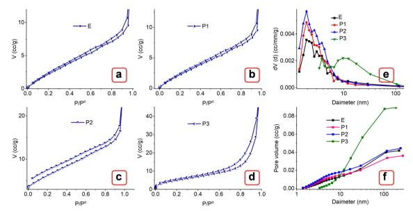
Fig. 3 N<sub>2</sub> adsorption curves of MOFs (a) E, (b) P1, (c) P2, (d) P3. BJH pore volume plots of MOFs (e) and (f).
