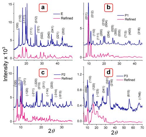
X-Ray diffraction patterns of MOFs (a) E, (b) P1, (c) P2, (d) P3, with corresponding refined curves and indexed miller indices.
