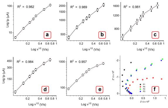
Corresponding calibration plots (a)–(e) of log of peak current ( $I_p$ ) vs. log of square root of scan rate ( $v^{1/2} V s^{-1}$ ). (f) Nyquist plots for P1, P2, P3, and P4.
