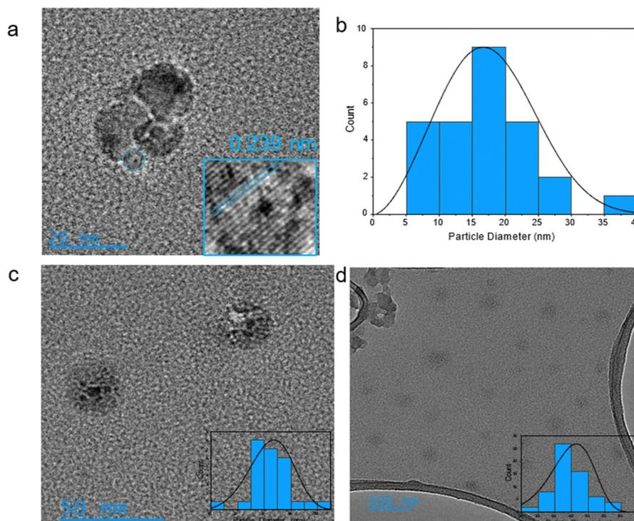
**Fig. 1** N-CPD samples were prepared for TEM by dispersion in IPA and sonication, before deposition on a carbon grid. (a) TEM image of 2H-CPD and (inset) magnification showing the crystal lattice grating, and (b) size-distribution from TEM analysis of 2H-CPD. TEM image and size distribution for (c) 4H-CPD and (d) 8H-CPD. The size distributions were determined from averaging all imaged N-CPDs.
