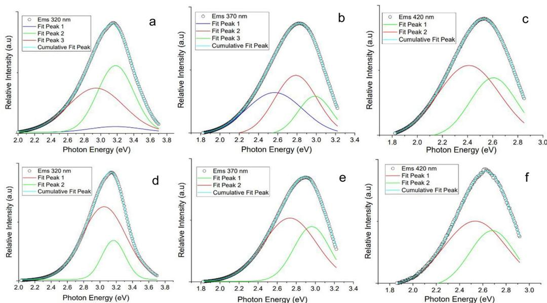
**Fig. 6** Gaussian peak fitting of photoluminescence data of 2H-CPDs synthesised from the 2H HTC of chitin-derived bio-oil, with excitation wavelengths of (a) 320 nm, (b) 370 nm, and (c) 420 nm. Gaussian peak fitting of photoluminescence data of the impurity fraction isolated after the 2 h HTC, with excitation wavelengths of (d) 320 nm, (e) 370 nm, and (f) 420 nm.
