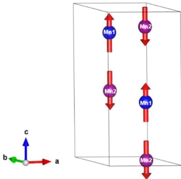
Fig. 5 Magnetic spin structure (red arrows) determined for  $\text{Mn}_2\text{Mo}_3\text{O}_8$  within the unit cell (black outline) at 10 K from the Rietveld refinement of powder neutron diffraction data. The blue and pink spheres represent manganese on the Mn1 (tetrahedral) and Mn2 (octahedral) crystallographic sites respectively.
