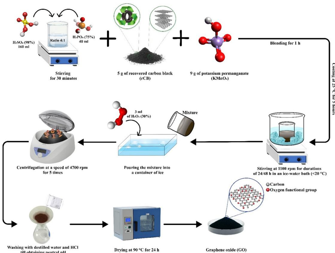
Fig. 1 Scheme of rCB-based GO synthesis through Hummers' method.
