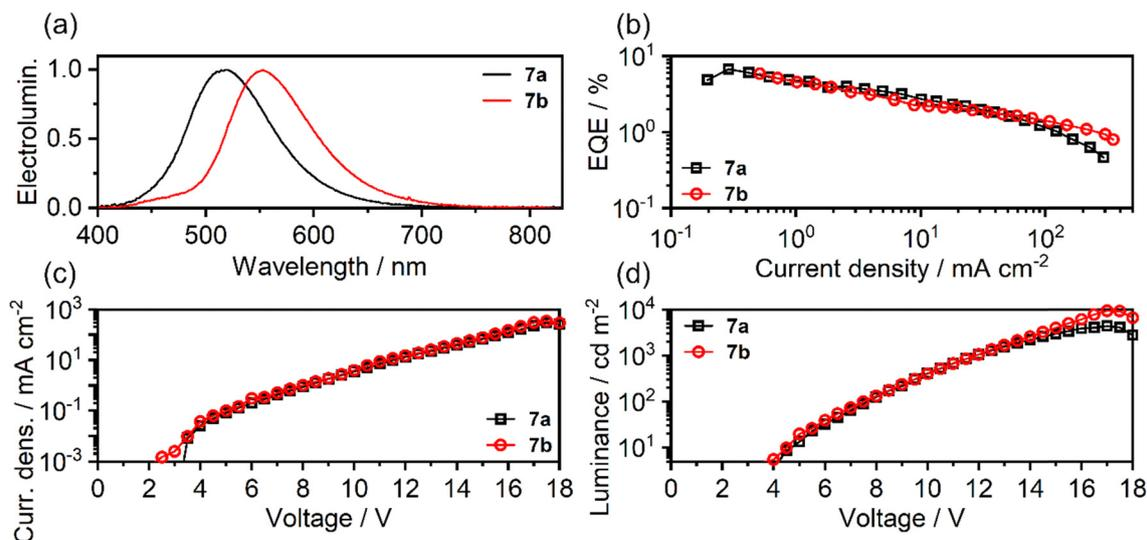
Fig. 7 Electroluminescent properties of OLEDs featuring **7a** and **7b** as emitters: (a) electroluminescence spectra; (b) EQE vs. current density; (c) current density vs. voltage; (d) luminance vs. voltage.
