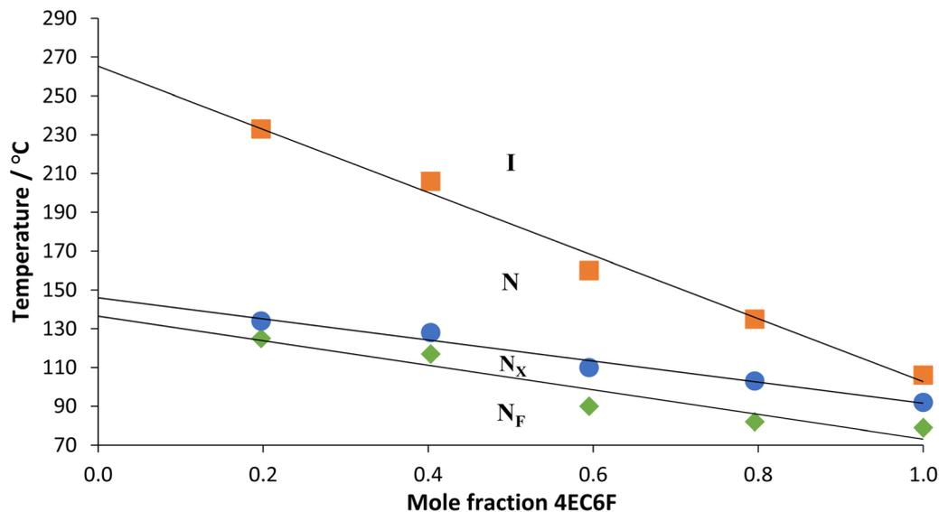
Fig. 5 Phase diagram constructed using binary mixtures of **EC1F** and **4EC6F**.<sup>47</sup> Squares denote  $T_{NI}$ , circles  $T_{N_xN}$  and triangles  $T_{N_FN_x}$ . The trendlines are shown for  $T_{NI}$ ,  $T_{N_xN}$  and  $T_{N_FN_x}$ .
