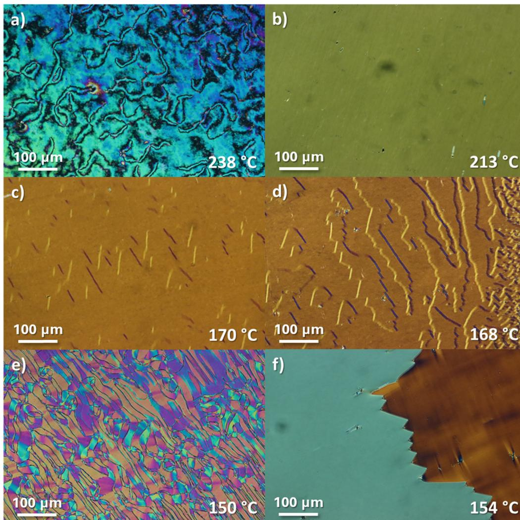
Fig. 4 Optical textures obtained for **EC2F** using polarised optical microscopy: (a) schlieren texture of the nematic phase seen for a sample sandwiched between untreated glass slides; the remaining textures were observed for samples in cells treated for planar anchoring, (b) uniform texture of the nematic phase, (c) and (d) chevron textures of the  $N_X$  phase, (e) banded texture of the ferroelectric nematic phase and (f) texture showing the twisted states of the ferroelectric nematic phase.
