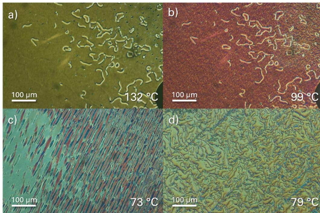
Fig. 7 Optical textures obtained using polarised light microscopy for a binary mixture composed of 40 mol% **EC2F** and 60 mol% **4EC6F** contained in a cell treated for planar alignment in (a) the N, (b) the  $N_X$ , and (c) the  $N_F$  phase. (d) The texture of the  $N_F$  phase obtained for a sample sandwiched between untreated glass slides.
