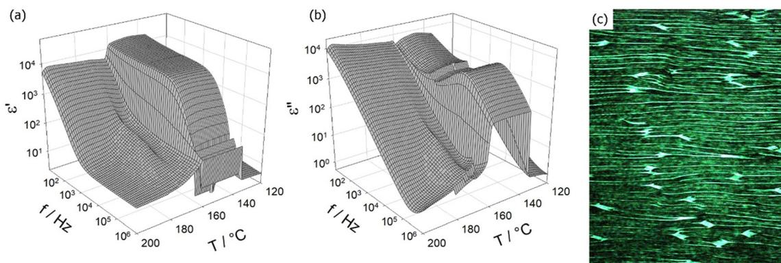
Fig. 10 (a) Real and (b) imaginary parts of the complex dielectric permittivity measured as a function of temperature and frequency for EC2F. (c) Image taken with an SHG microscope in the ground state (no applied voltage)  $N_F$  phase (at 155 °C) for a sample prepared in a cell with planar anchoring. Incident IR radiation caused strong emission of double-frequency (green) light.
