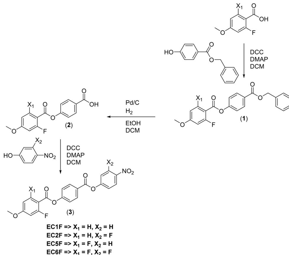
Scheme 1 Synthetic route used to prepare EC1F, EC2F, EC5F and EC6F.
