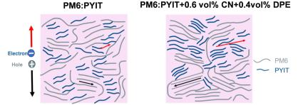
Hypothetical diagram of changes in morphology and molecular aggregation state of the active layer
