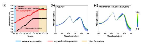
Fig. 6 (a) The absorption peak position of PYIT as a function of time. In situ absorption spectra of binary films (b) without additives and (c) with dualadditive during the film-formation process
