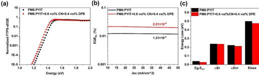
Fig. 3 (a) FTPS-EQE spectra; (b) EQE<sub>EL</sub> spectra and (c) energy loss data of the PM6:PYIT devices before and after dual-additive treatment.
