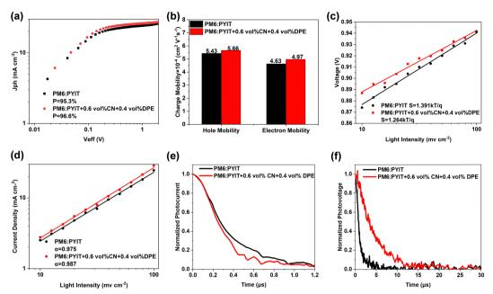
Fig. 2 (a)  $J_{\rm ph}$  versus  $V_{\rm eff}$  of the devices. (b) Hole mobility and electron mobility of the devices. (c)  $J_{\rm SC}$  and (d)  $V_{\rm OC}$  dependence on the light intensity of OSCs. Normalized (e) TPC and (f) TPV data for the devices
