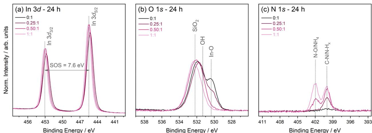
Fig. 3 XPS core level spectra, including (a) In 3d, (b) O 1s, and (c) N 1s, for each stabiliser ratio after 24 hours. Spectra are normalised to the respective areas of the In  $3d_{5/2}$  peak.
