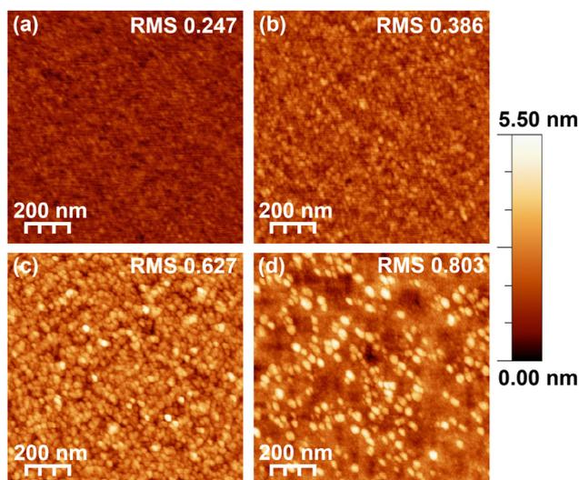
Fig. 6 AFM images ( $1 \times 1 \mu\text{m}^2$ ) of the four annealed In<sub>2</sub>O<sub>3</sub> films with varying stabiliser concentrations: (a) 0, (b) 0.25, (c) 0.50 and (d) 1. The corresponding RMS values in nm are shown in the upper right corner of each image. All images are shown over the same height range.
