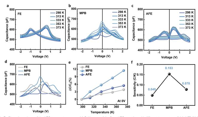
Fig. 3 Phase dependency of the HZO temperature sensor. (a) C-V curves of the 6 nm HZO capacitor with different temperatures ((a) 1:1 FE, (b) 1:2 MPB, (c) 1:3 AFE). (d) C-V curves of different phases at room temperature. (e)  $\Delta C/C_0$  percentage as a function of the temperature for different phase samples. (f) Temperature sensitivity of the different phase samples.
