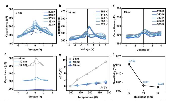
Fig. 4 Thickness dependency of the HZO temperature sensor. (a) C-V curves of the MPB HZO capacitor with different temperatures ((a) 6 nm, (b) 10 nm, (c) 15 nm). (d) C-V curves of different thicknesses at room temperature. (e)  $\Delta C/C_0$  percentage as a function of the temperature for different thickness samples. (f) Temperature sensitivity of the different thickness samples.
