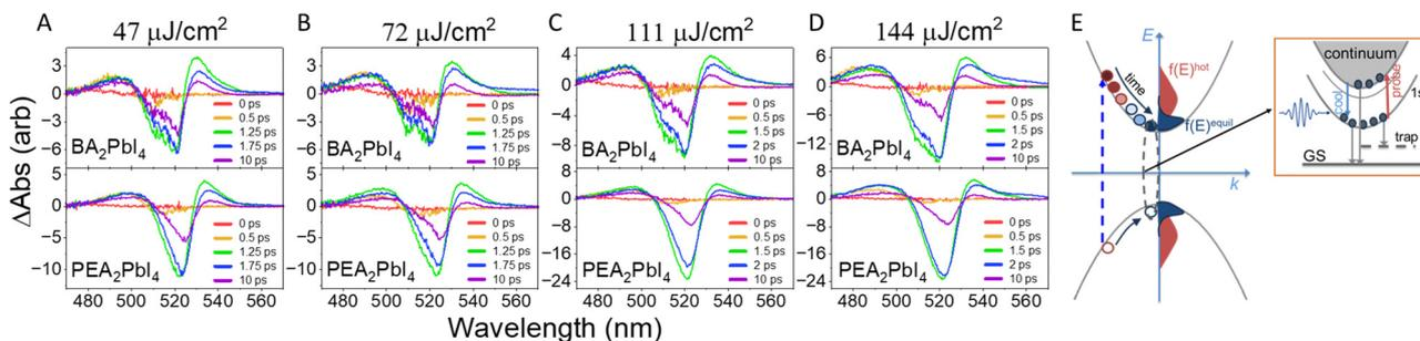
Fig. 3 Transient absorption spectra as function of pump fluence. The 8-panel figure shows the differential absorption spectra for BA<sub>2</sub>PbI<sub>4</sub> (top) and PEA<sub>2</sub>PbI<sub>4</sub> (bottom) at four pump fluences (A) 47 μJ cm<sup>-2</sup>, (B) 72 μJ cm<sup>-2</sup>, (C) 111 μJ cm<sup>-2</sup>, and (D) 144 μJ cm<sup>-2</sup>. (E) Schematic of the photoexcitation process. The inset shows a two-particle representation of the excitonic process.
