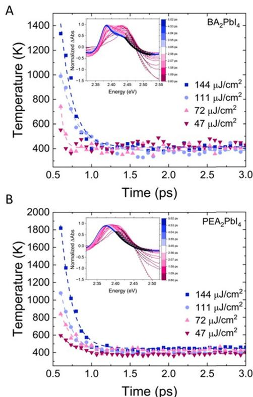
Fig. 5 Photoexcited carrier cooling. (A) and (B) Transients of cooling curves (carrier temperature), obtained from eqn (4), for all pump fluences for  $\text{BA}_2\text{PbI}_4$  and  $\text{PEA}_2\text{PbI}_4$ , respectively. The dashed lines show fits for an exponential decay in each case. The insets show the normalized TA signal at different time-slices distinguished by different colours and the high-energy tail fits using eqn (4) are shown by dashed black lines.
