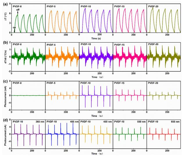
Fig. 4 Comparative analyses of photo-induced temperature variation and pyroelectric current of different films. (a) Temperature changes ΔT, (b) temperature change rate dT/dt and (c) photo-pyroelectric currents  $I_{py}$  of different films under periodic 365 nm LED light irradiation of 100 mW cm<sup>-2</sup>, tested by a thermocouple module. (d) Photo-pyroelectric response of PVDF-10 films under light with different wavelengths
