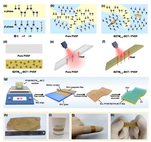
Fig. 1 Scheme design, preparing processes and exhibition of the PVDF-x composite films. (a-f) Schematic diagram enhancing the polar phase content (a-c) and photo-absorption (d-f) by adding BZTM0.12-BCT particles into PVDF. (g) Preparation processes of the PVDF-x composite films. (h-k) Measurement of the (h) size, (i) and (j) flexible properties and (k) tearing resistance performance of PVDF-x composite films.
