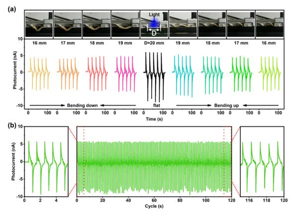
Fig. 6 Stability measurements of the photo-pyroelectric currents of the PVDF-10 film. The used light is a 365 nm LED with a light intensity of 100 mW cm<sup>-2</sup>. (a) Top photos present the PVDF-10 films with different degrees of bending. The bottom curves are the photo-pyroelectric current corresponding to the top bending films. (b) Cycling stability of the PVDF-10 film under periodic light illumination
