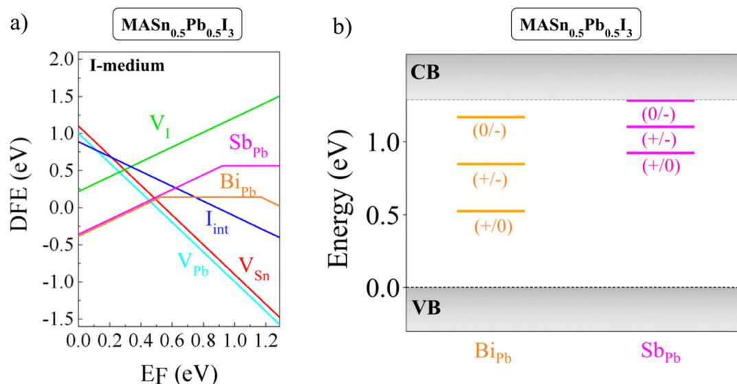
Fig. 2 (a) Defect formation energies of substitutional Bi<sub>Pb</sub> and Sb<sub>Pb</sub> dopants compared with the more stable native defects in MAPb<sub>0.5</sub>Sn<sub>0.5</sub>I<sub>3</sub> (I-medium conditions); (b) associated thermodynamic ionization levels. Defect quantities have been calculated at PBE0-SOC ( $\alpha = 0.20$ ) level of theory by including DFT-D3 dispersions.
