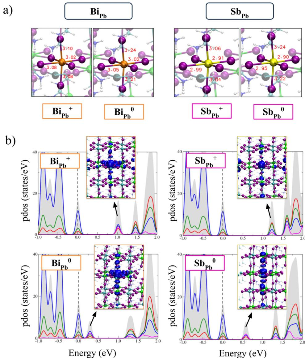
Fig. 3 (a) Equilibrium structures of the positive and neutral Bi<sub>Pb</sub>, Sb<sub>Pb</sub> defects; (b) atom-projected density of states (PDOS) of the same defects, highlighting the presence of deep trap states in the band gap of the perovskite (blue = I, red = Pb, green = Sn, purple = dopant). In the diagrams the VBM energy is set to zero (dotted line). In the insets the plots of the LUMO (HOMO) Kohn–Sham (KS) orbitals of the positive (neutral) defects are reported.
