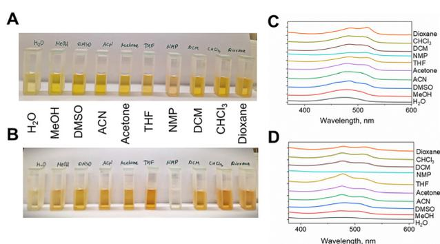
**Fig. 1** Solvent-dependent colour change of PETH (A) and qH-PETH (B) solutions in selected solvents at identical concentration (0.75 mg mL<sup>-1</sup>) and UV-vis absorbance spectra of PETH (C) and qH-PETH (D) in different solvents.
