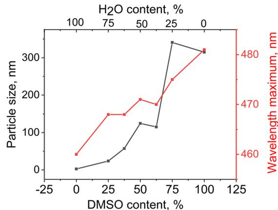
Fig. 3 Dependence of particle size (black) and UV-vis absorption maximum (red) of the qH-PETH in DMSO/water mixtures ( $0.25 \text{ mg mL}^{-1}$ ).
