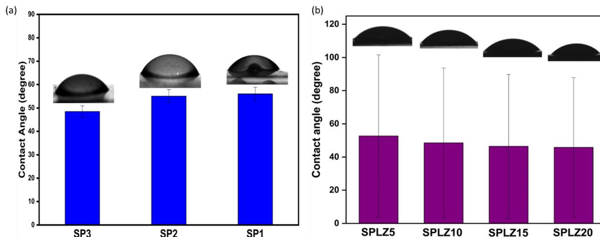
Fig. 14 Water contact angle measurements of (a) SA/PVP films with different weight percentage ratios (90 : 10, 80 : 20, and 70 : 30) and (b) SA/PVP/Lap-Zr-MOF with different weight percentages (5%, 10%, 15%, and 20%).
