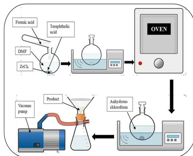
Fig. 1 Synthesis of Zr–metal organic framework (UiO-66).
